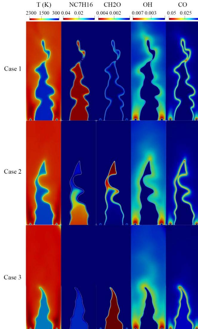
Figure 5. The instantaneous distributions of temperature, mass fraction of  $\text{NC}_7\text{H}_{16}$ ,  $\text{CH}_2\text{O}$ ,  $\text{CO}$  and  $\text{OH}$  (from left to right column) in Cases 1-3 (CF, transition from CF to LTI, and LTI regimes), respectively.
