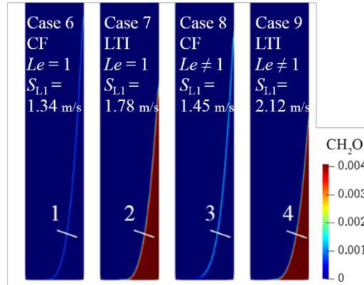
Figure 6. CH<sub>2</sub>O mass fraction distribution of 2DLF for Cases 6-9.
