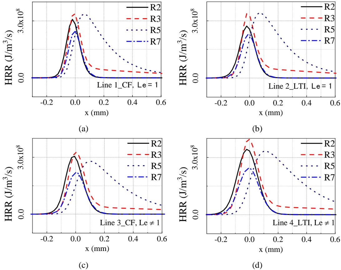
Figure 8. Spatial distribution of HRR from key elementary reactions for Cases 6-9, along the reaction path  $\text{CH}_2\text{O}\rightarrow\text{HCO}\rightarrow\text{CO}\rightarrow\text{CO}_2$ .
