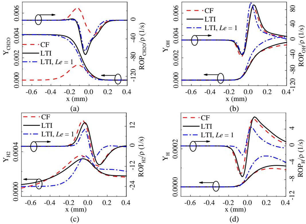
Figure 9. Species mass fractions and ROPs of CH<sub>2</sub>O (a), OH (b), H<sub>2</sub> (c) and H radicals (d) along Line 2 (LTI,  $Le = 1$ ), Line 3 (CF) and Line 4 (LTI).
