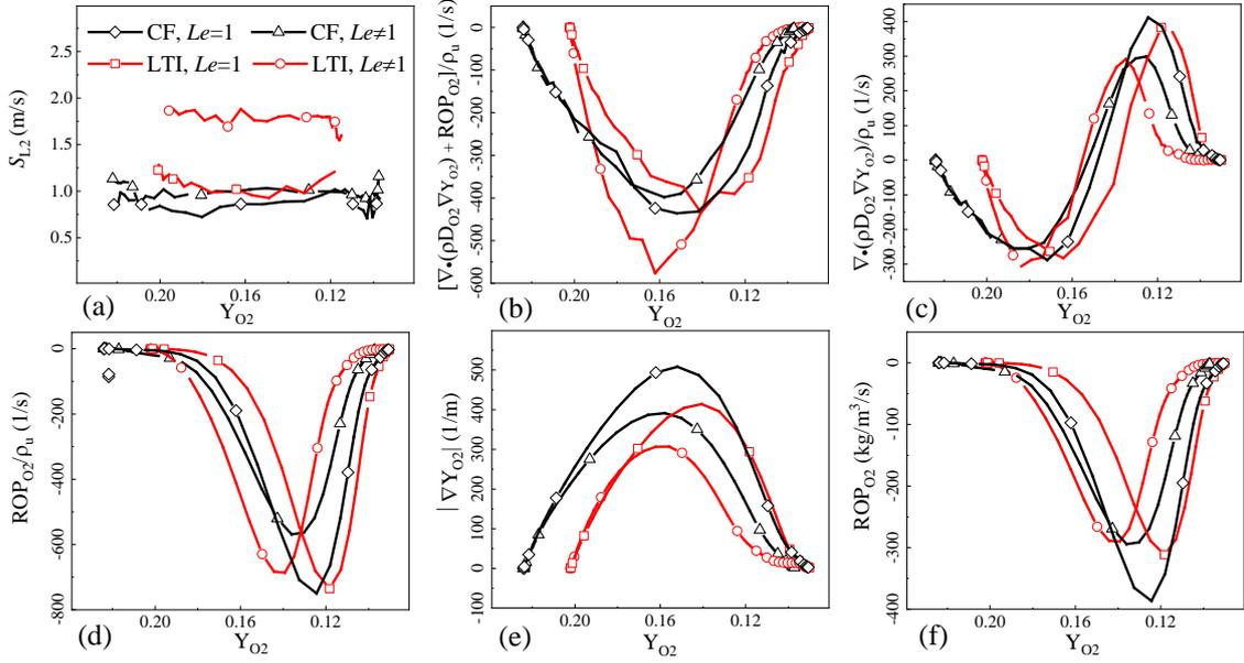
Figure 10.  $S_{L2}$  (a), the budget terms of  $S_{L2}$  (b, c, d),  $|\nabla Y_{O_2}|$  (e) and  $ROP_{O_2}$  (f) as a function of  $Y_{O_2}$  along Lines 1 (CF,  $Le = 1$ ), 2 (LTI,  $Le = 1$ ), 3 (CF,  $Le \neq 1$ ) and 4 (LTI,  $Le \neq 1$ ). The unburnt mixture density ( $\rho_u$ ) in LTI case is 0.423 kg/m<sup>3</sup> and in CF case is 0.517 kg/m<sup>3</sup>.
