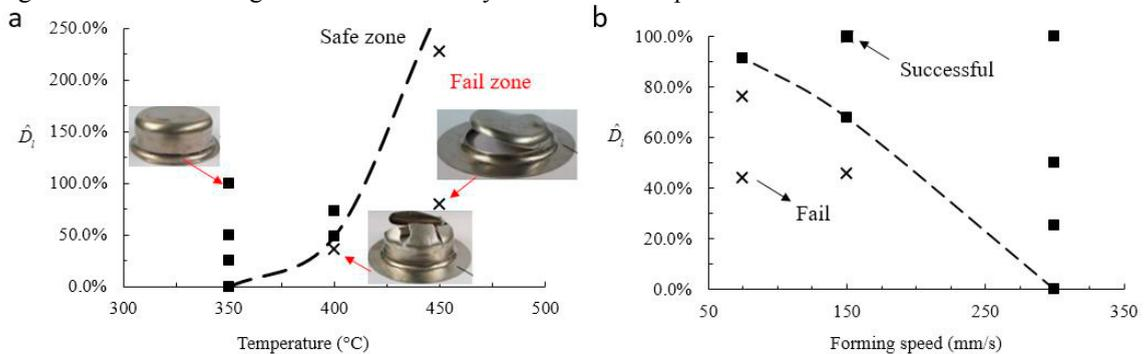
Fig. 5. (a) Temperature effect; (b) Forming speed effect
