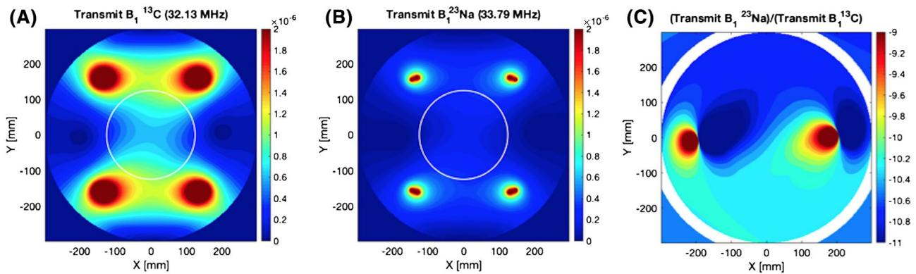
**FIGURE 3** Simulated transmit  $B_1$  field distributions for the transmit volume coil used in this study. Transmit  $B_1$  distribution at  $^{13}\text{C}$  (32.13 MHz) and  $^{23}\text{Na}$  (33.79 MHz) frequencies (A and B, respectively). (C) Ratio between required power for 90-degree flip for  $^{13}\text{C}$  and  $^{23}\text{Na}$  frequencies for the same coil. The phantom position is highlighted with a white line
