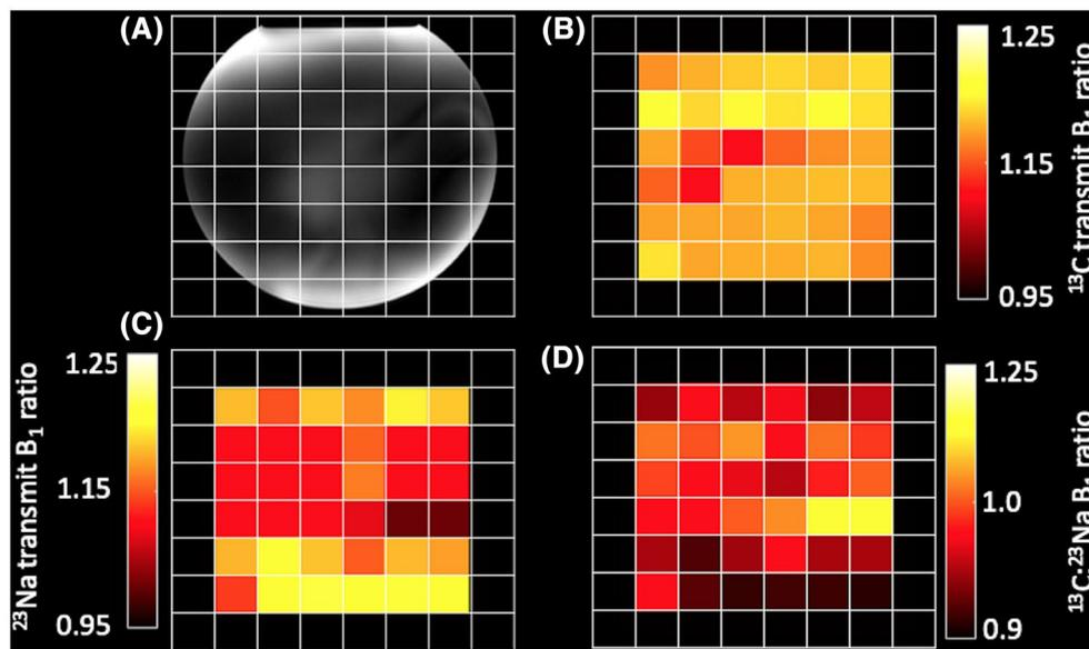
**FIGURE 4** (A) Chemical shift image grid overlaid on an 8 L phantom containing 150 mmolL<sup>-1</sup> NaCl and 102 mmolL<sup>-1</sup>  $^{13}\text{C}$ -pyruvate. (B and C)  $^{13}\text{C}$  and  $^{23}\text{Na}$  transmit  $B_1$  maps, respectively. (D) Ratiometric difference maps between B and C
