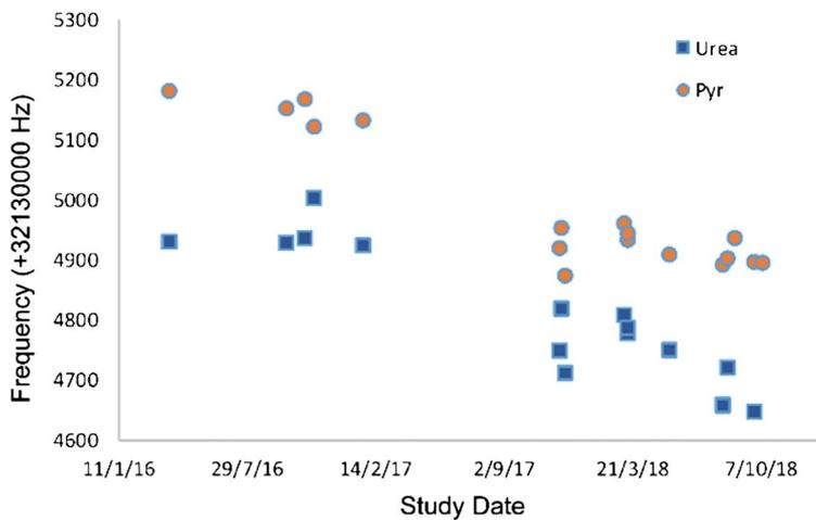
**FIGURE 6** Measured frequency (+32130000 Hz) of  $^{13}\text{C}$ -pyruvate (pyruvate) in vivo and  $^{13}\text{C}$ -urea in vitro for all human brain hyperpolarization studies at site B over a 31-month period
