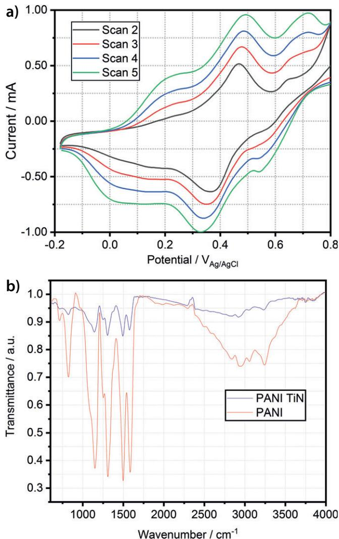
Fig. 1 (a) CV cycle of a  $0.1M$  polyaniline and  $0.1\ g\ L^{-1}$  solution at room temperature (approx.  $25\ ^\circ C$ ). (b) FTIR spectrums of 25 cycle PANI and PANI TiN samples.
