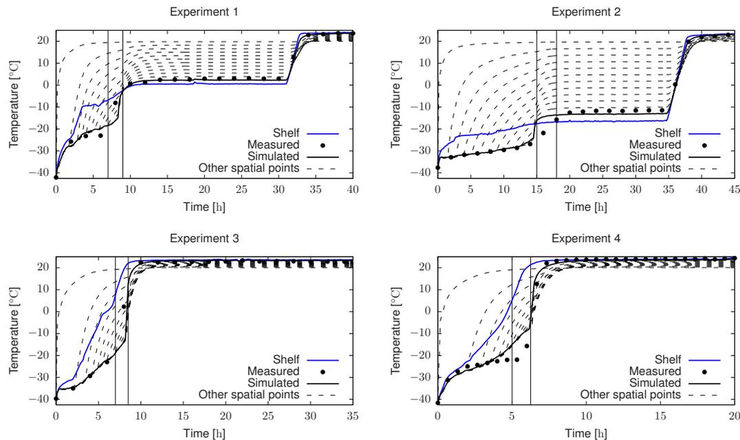
**Figure 3.** Predictive capabilities of the freeze-drying model from the product temperature point of view. Blue line corresponds to the shelf temperature. Continuous black line and black dots represent, respectively, the model predictions and experimental measurements at the bottom of the product. Dashed black lines correspond to the model prediction at other spatial points in the product. Vertical lines represent the end of primary drying and the beginning of secondary drying.
