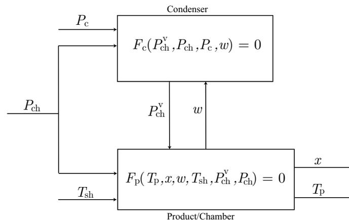
**Figure 2.** Schematic representation of the freeze drying process. Two subsystems are considered, the condenser and the product. The arrows entering the subsystems represent the process control variables whereas output arrows represent the state variables.
