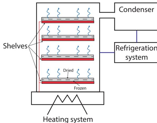
**Figure 1.** Schematic representation of the lyophilization pilot plant.
