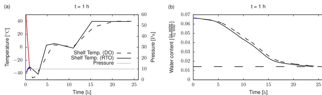
**Figure 7.** Comparison, in terms of process duration, between the RTO approach (continuous black lines) and the off-line control profile (dashed black lines). (a) Shelf temperature and chamber pressure. (b) Mean water content evolution. Blue and red segments in subplot (a) correspond with the real plant measurements for shelf temperature and chamber pressure, respectively.
