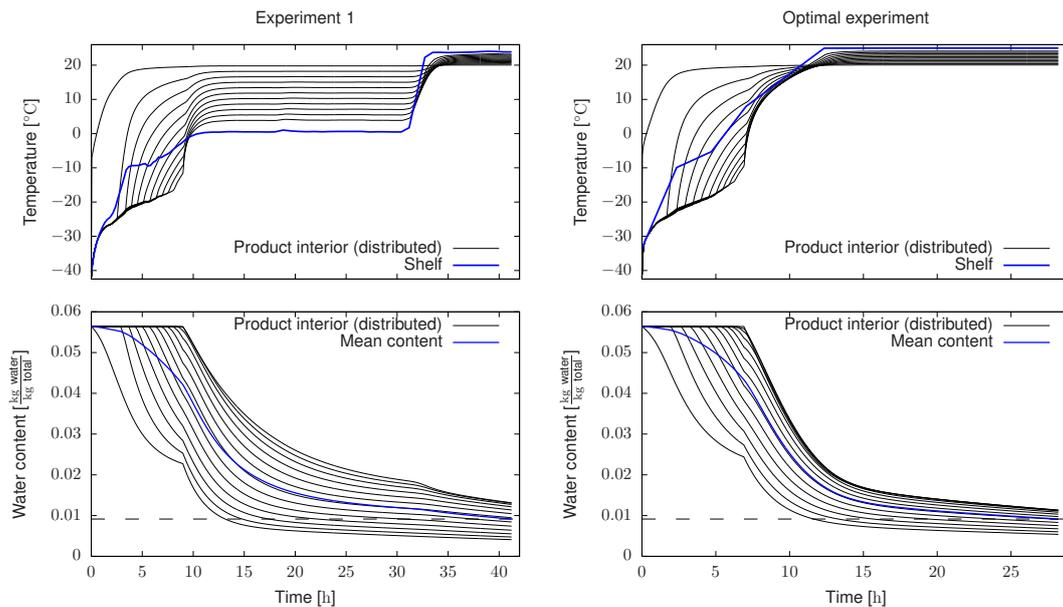
**Figure 5.** Evolution of the product temperature and shelf temperature (top figures) as well as water content (bottom figures). Figures on the left correspond with experiment 1 whereas the optimal design results are represented on the figures on the right. Horizontal line on the bottom figures represent the constraint on the final water content.
