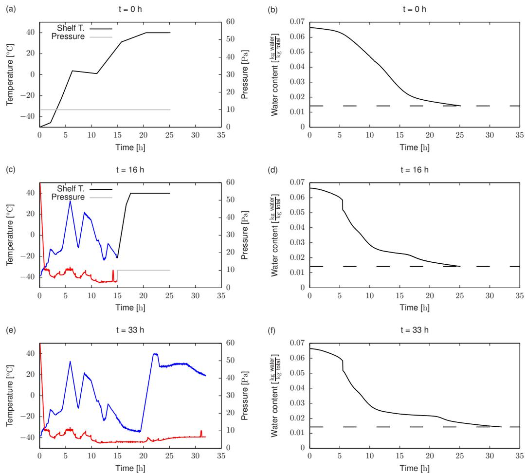
**Figure 6.** Offline and real time optimization (RTO) scheme results. Subfigures (a,c,e) represent the evolution of shelf temperature (decision variable) and chamber pressure. Black and gray parts of the profiles correspond with the optimal solution. Blue and red parts correspond with the plant measurements. Subfigures (b,d,f) represent the evolution of product mean water content. Dashed line indicates the quality objective to reach.
