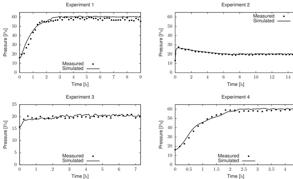
**Figure 4.** Predictive capabilities of the freeze-drying model for the chamber vapor pressure. Black circles represent the chamber vapor pressure obtained from measurements of Pirani and total chamber pressure whereas continuous black lines correspond to the model predictions.
