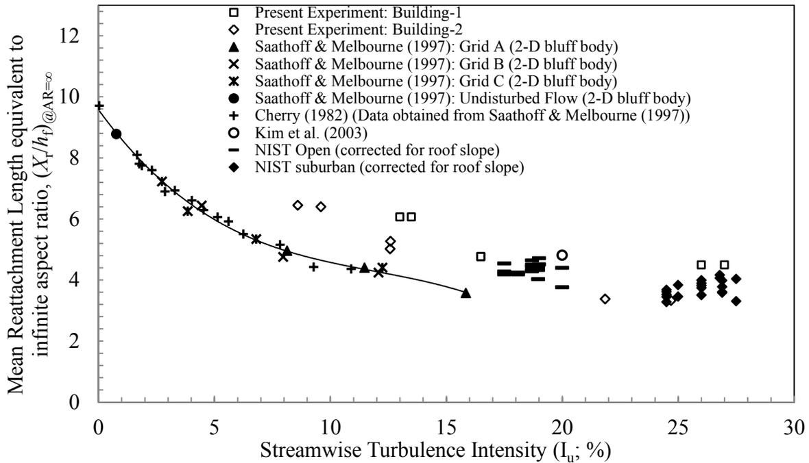
Figure 10: Variation of mean reattachment length, corrected to infinite aspect ratio,  $(X_r/h_f)_{@AR=\infty}$ , as a function of streamwise turbulence intensity. A polynomial fit through the 2D bluff-body data is also shown for clarity.
