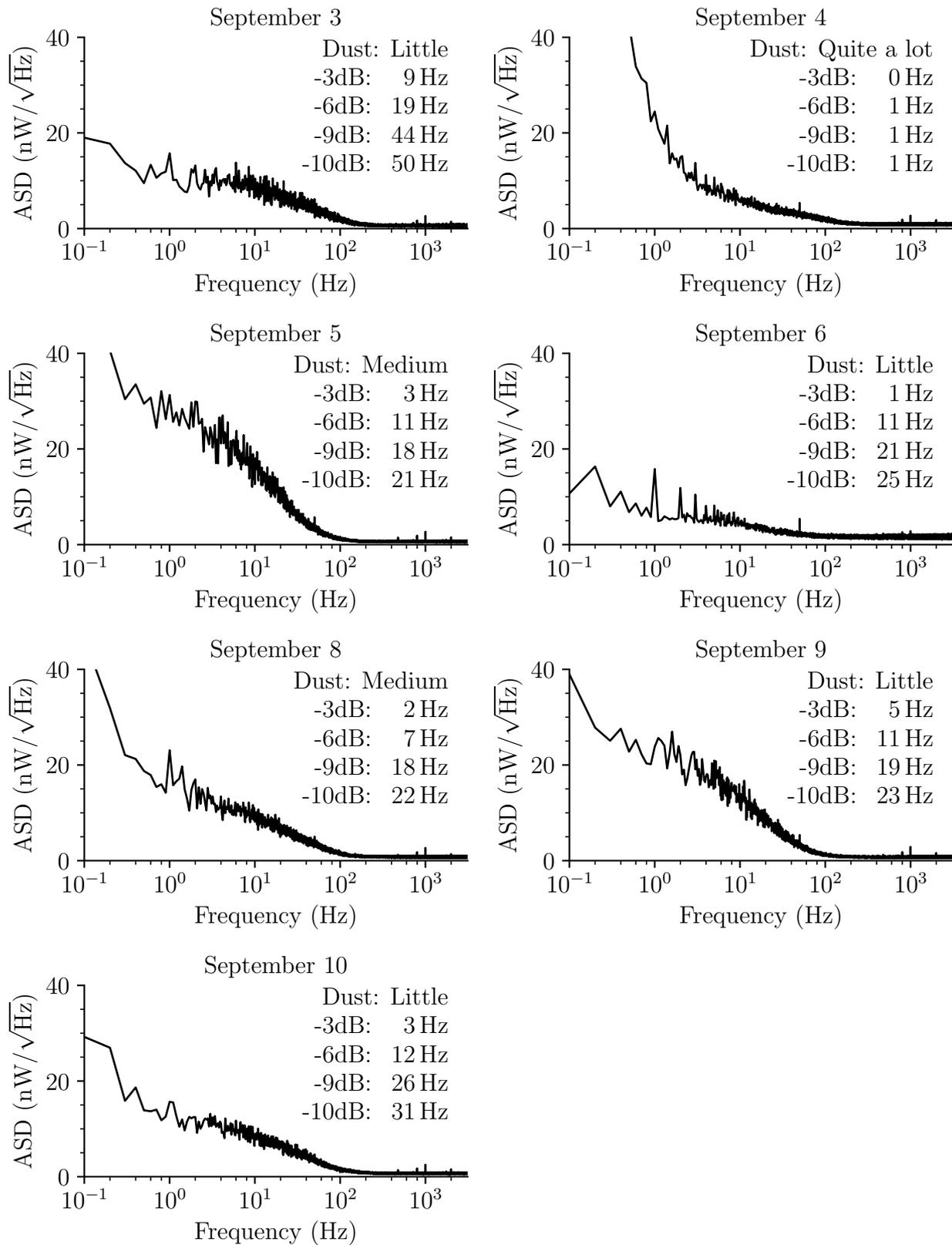
**Figure 3.** Daily scintillation measurements collected during 2017 September, using the technique described in Section 3. The qualitative dust levels are described in Table 1. The absolute values for September 6 are low due to a temporary change in collection optics.
