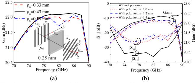
Fig. 3 Analysis of the  $45^\circ$  linear polarizer. (a) Simulated peak gain with different periods  $p_6$ ; (b) Simulated peak gain and  $|S_{11}|$  with and without the polarizer.
