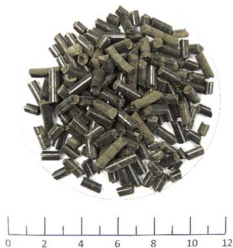
**Figure 5.** Feedstock sewage sludge pellets, scale size in cm.
