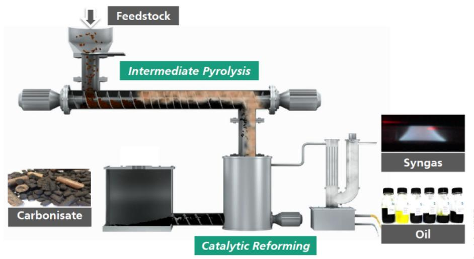
**Figure 1.** Schematic principle of the TCR<sup>®</sup> process<sup>30</sup>.
