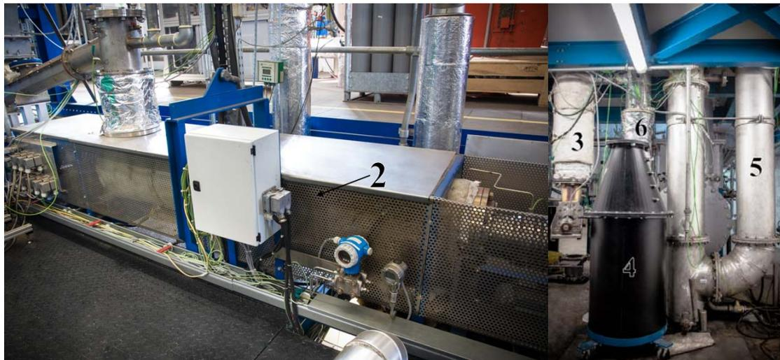
**Figure 4.** TCR<sup>®</sup> 30 (pilot scale) – maximum capacity 30kg/hr. 1) Sludge system, 2) Reactor, 3) Post-reformer, 4) Solid particle container, 5) Gas cooler/condenser, 6) Cyclone.
