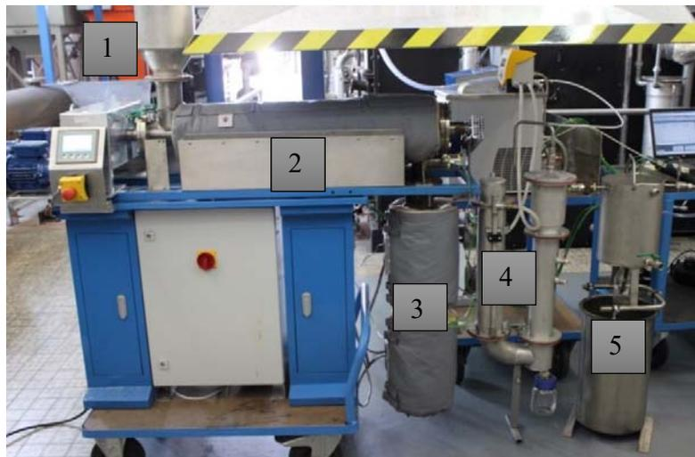
**Figure 3.** TCR<sup>®</sup> 2 (Lab scale) – maximum capacity 2kg/hr. 1) feed hopper, 2) reactor, 3) post-reformer, 4) gas cooler/ condenser #1, 5) gas cooler/condenser#2
