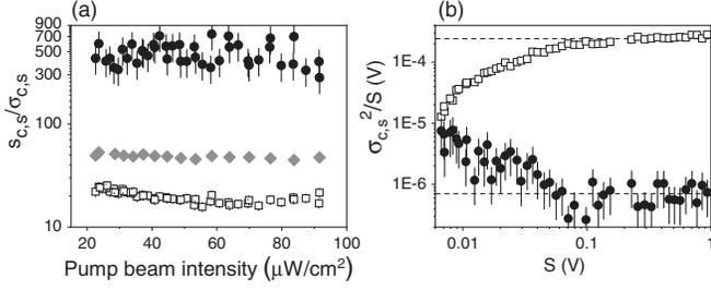
FIG. 4. (a) Signal-to-noise ratio of the signal quadratures measured for  $\omega_M = 2\omega_L$  as a function of the pump beam intensity. The out-of-phase quadrature (closed dots) shows an improved SNR with respect to the in-phase quadrature (open squares), and to the case of no modulation (gray diamonds). (b) Corresponding noise scaling with signal amplitude.
