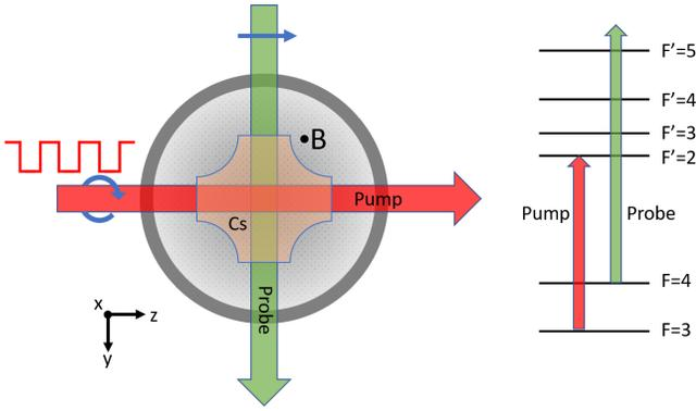
FIG. 1. Schematics of the apparatus: a circularly polarized amplitude-modulated pump beam creates atomic coherences in the ground states of the Cs atoms by resonant ( $F = 3$ ) and indirect pumping ( $F = 4$ ). The generated collective atomic spin precesses orthogonally to the applied static magnetic field. A linearly polarized probe beam is used to extract information on the atomic precession via Faraday-like, nondestructive measurements.
