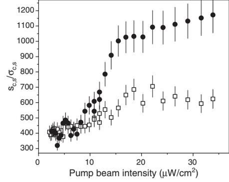
FIG. 5. Signal-to-noise ratio of a Bell-Bloom magnetometer, as a function of the pump beam intensity. Similar to the case of modulation at  $2\omega_L$ , the out-of-phase quadrature (closed dots) is increased with respect to the in-phase quadrature (open squares) for intensities larger than roughly  $15 \mu\text{W}/\text{cm}^2$ . Note that, as expected, the overall magnetization is higher when hitting the Bell-Bloom resonance with respect to other modulation frequencies.
