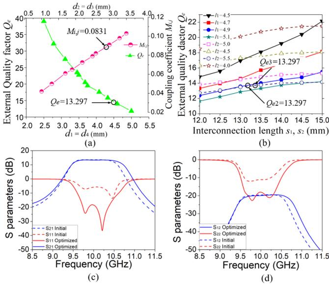
Fig. 4. (a) External quality factor  $Q_e$  versus dimension  $d_1, d_4$ ; Coupling coefficient  $M_{i,j}$  versus dimension  $d_2, d_3$ . (b) External quality factor  $Q_e$  versus dimension  $s_1, s_2$ . (c) Simulation response with initial and optimized values  $S_{11}$  and  $S_{21}$ . (d)  $S_{22}$  and  $S_{12}$ .
