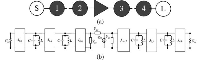
Fig. 1. Topology and equivalent circuit of the transistor with input and output resonator matching. (a) Schematic representation of the circuit. (b) Lumped circuit model.  $G_S$  and  $G_L$  are the source and load conductance;  $Y_{gs}$ ,  $Y_{ds}$ , and  $Y_{ds}$  are the admittances between transistor's gate, source and drain;  $g_m$  is the transconductance.
