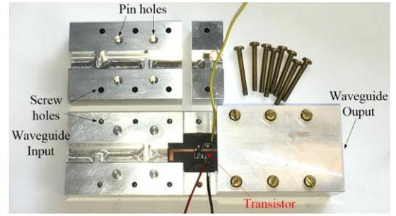
Fig. 5 Photograph of the fabricated waveguide filter-amplifier device.
