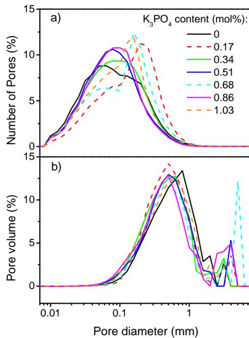
**Fig. 2.** Distribution of pore size (equivalent sphere diameter) of glass foams with different  $K_3PO_4$  content (XMT data). a) Number of pores with bimodal distributions shown as dashed lines and b) pore volume. The pore diameter is in log space.
