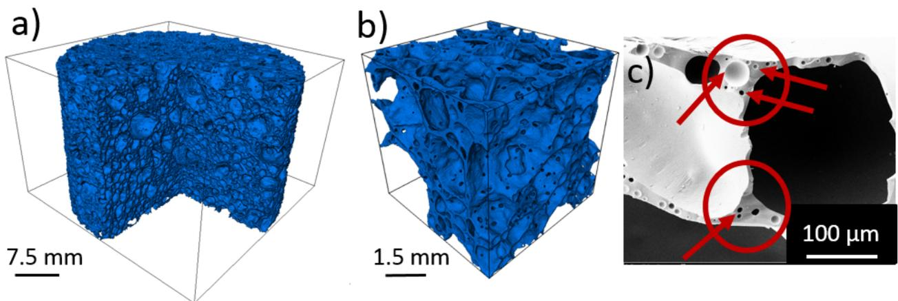
**Fig. 1.** 3D micrographic reconstructions of the pore structure of glass foam prepared without  $\text{K}_3\text{PO}_4$  in a) full-size, b) subvolume, and c) SEM secondary electron image of struts (marked by circles), pore walls, and small pores inside struts (marked by arrows).
