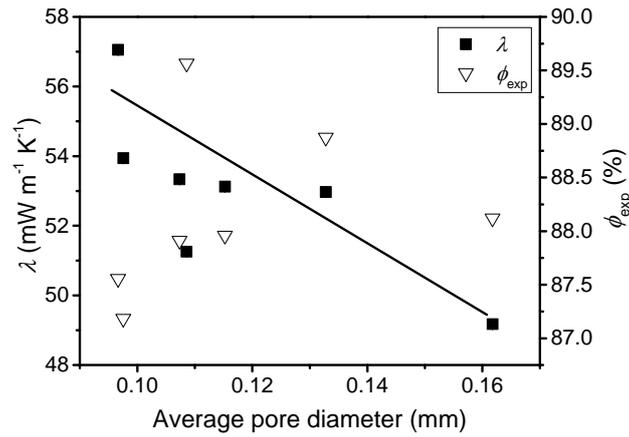
**Fig. 4.** Change in thermal conductivity ( $\lambda$ ) and porosity ( $\phi_{exp}$ ) with increasing average pore diameter based on  $D_{eq}$ . Errors of  $\lambda$  and  $\phi_{exp}$  are  $0.1 \text{ mW m}^{-1} \text{ K}^{-1}$  and 0.1 point, respectively. The error of pore diameter is  $\pm 0.1 \text{ mm}$ . The line is intended as visual guideline.
