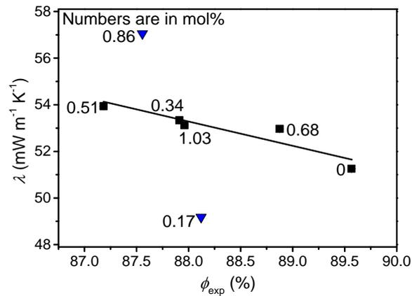
**Fig. 3.** Change in thermal conductivity ( $\lambda$ ) with the porosity ( $\phi_{\text{exp}}$ ). The labels refer to the  $\text{K}_3\text{PO}_4$  content. Outliers are marked with triangles. The errors are smaller than the symbols. The line is a visual guideline.
