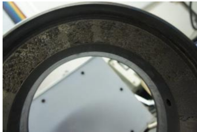
Figure 10: Spalling on the outer race
