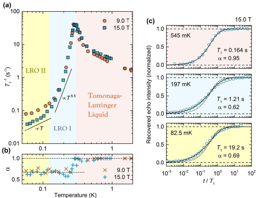
FIG. 3. (a)  $^{14}\text{N}$  NMR relaxation rate  $T_1^{-1}$  as a function of temperature in 9.0 T and 15.0 T. (b) Temperature evolution of the stretch exponent  $\alpha$  in the relaxation function. (c) Nuclear magnetization recovery curves for 15 T at 545 mK, 197 mK, and 82.5 mK, from upper to lower panels. Solid lines are fits using the theoretical relaxation function with varying  $\alpha$  while dotted lines are with  $\alpha = 1$  for comparison.
