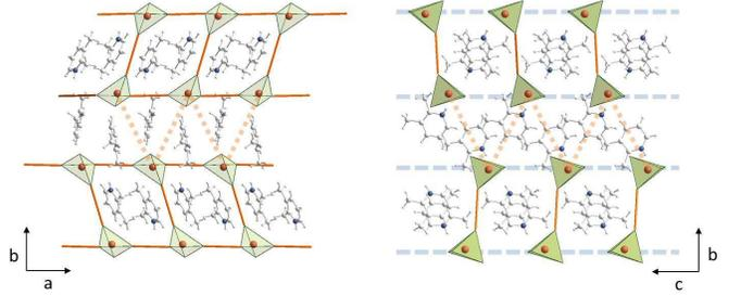
FIG. 1. Crystal structure of DIMPY where orange balls in green tetrahedra represent spin-1/2 Cu ions of  $\text{CuBr}_4$  units and solid lines represent predominant exchange pathways forming a ladder-like network. Broken lines represent much weaker couplings between the ladders. (a) View presenting the ladders side by side. (b) View along the ladder direction showing the coupling of the ladders along the  $b$  and  $c$  axes.
