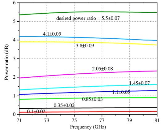
Fig. 12. Simulation power ratios of the nine types of power dividers.
