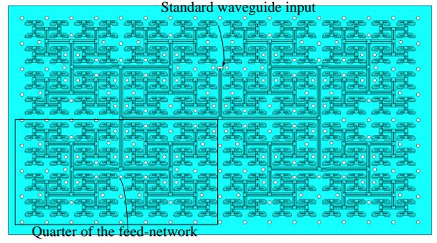
Fig. 7. 16x32 full-corporate single ridge-waveguide feed network.
