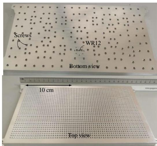
Fig. 13. Photo of the fabricated antenna array.
