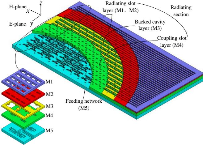
Fig. 1. Configuration of the 32×64-slot antenna array.
