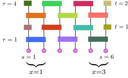
FIG. 1. Structure of the local unitary circuits studied in this paper. The on-site Hilbert space dimension is  $q$ . Each two-site gate is a  $q^2 \times q^2$  unitary matrix. For the random circuit model of Eq. (4), each gate is randomly chosen from the Haar distribution. For the Floquet models considered in Secs. IV and V, the two-site gates are defined by the Floquet unitaries in Eqs. (28) and (33), respectively.
