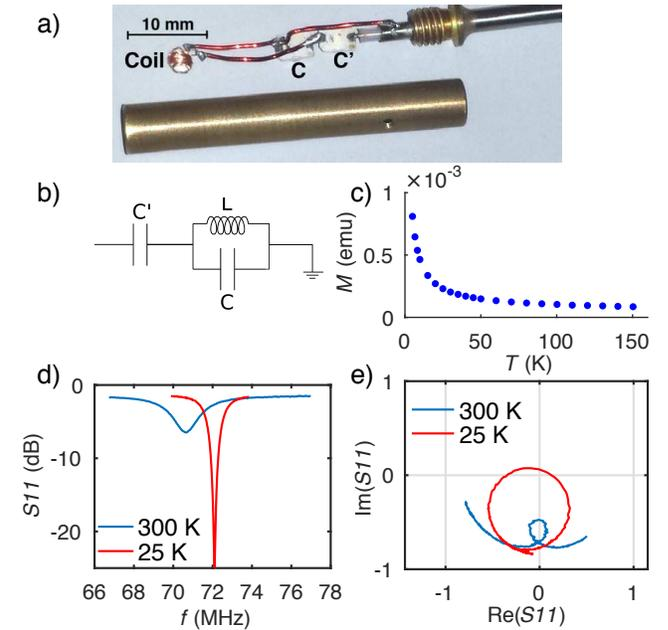
FIG. 1. (a) Photograph of the NMR circuit and protective can. (b) NMR circuit diagram. (c) Magnetic moment of a chip capacitor as a function of  $T$ . (d) Resonance of the circuit at 300 and 25 K as observed in  $S_{11}$  and (e) its polar plot.
