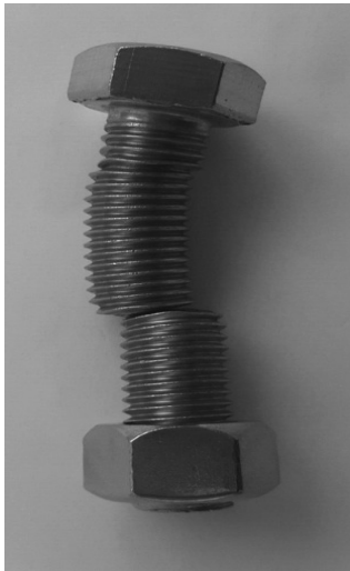
Fig.3 Load-deflection curve and failure mode of M16 bolt Grade A4-80 loaded in double shear.
