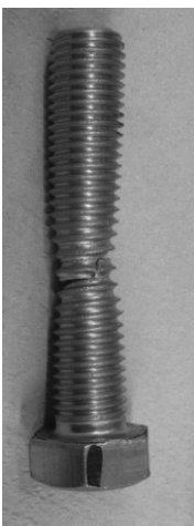
Fig.4 Load-elongation curve and failure mode of M16 bolt Grade A4-80 loaded in tension.
