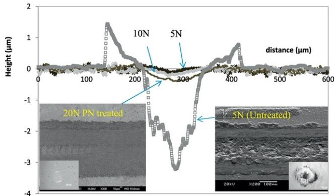
Figure 9. Fig. 9 Wear tracks for the untreated and PN treated (720/25) samples at different loads and the SEM images of the wear track of untreated sample under a load of 5 N and the scar on the  $\text{Al}_2\text{O}_3$  ball, and the wear track of the PN treated sample (720/25) under a load of 20 N and the scar on the  $\text{Al}_2\text{O}_3$  ball.
