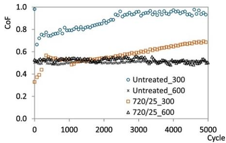
Figure 10. Coefficient of friction comparison of untreated and PN treated (720/25) samples under elevated temperatures of 300 °C and 600 °C.
