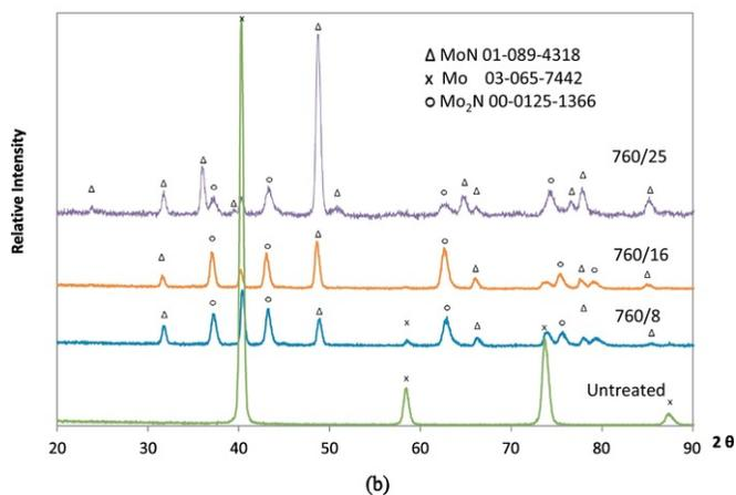
Figure 5. Fig. 5 Phase constituent changes with (a) temperature (25 h) and (b) treatment time (760°C).
