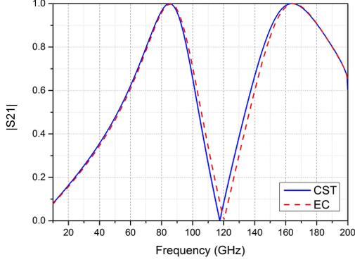
Fig. 2. Transmission coefficient versus frequency under normal incidence for a free-standing FSS with the following geometrical parameters:  $x$ -period,  $d_x = 1.5$  mm;  $y$ -period,  $d_y = d_x$ ; inner radius of the first aperture,  $a_1 = 0.3$  mm; outer radius of the first aperture,  $b_1 = 0.4$  mm; inner radius of the second aperture,  $a_2 = 0.55$  mm; outer radius of the second aperture,  $b_2 = 0.65$  mm.
