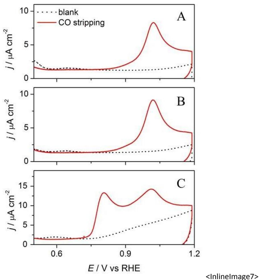
**Figure 5: Voltammetric profiles in 0.5 M H<sub>2</sub>SO<sub>4</sub> for the oxidation of a CO monolayer on the Pt-modified gold electrodes prepared at (A) 1.06 V vs RHE, (B) 0.75 V vs RHE, (C) 0.65 V vs RHE; scan rate: 0.02 V s<sup>-1</sup>.**
