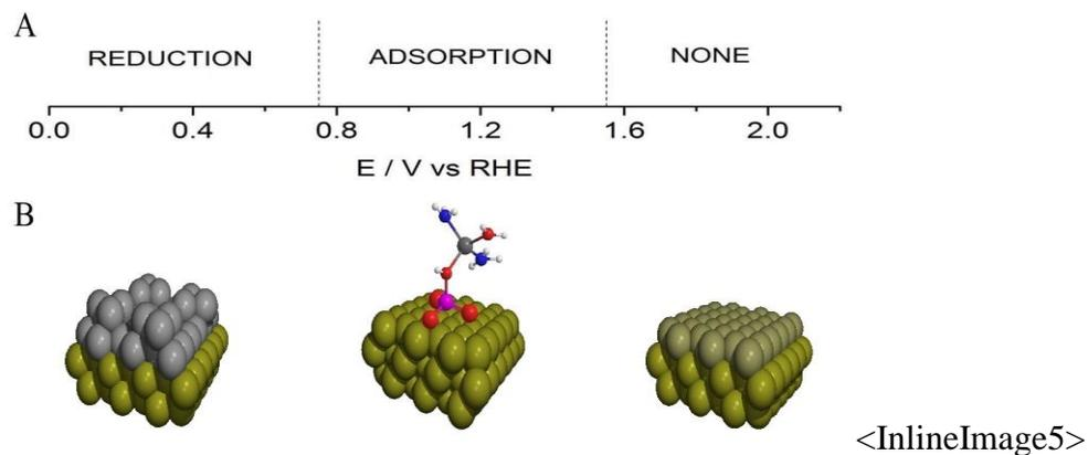
**Figure 4: (A) Scheme of the potential-dependence for the phosphate-mediated adsorption of cisplatin on Au polycrystalline electrode. (B) Hard-sphere model corresponding to the phenomena observed at the range of potentials. Yellow spheres stand for gold, grey spheres stand for platinum, pale yellow spheres stand for gold oxide layer.**
