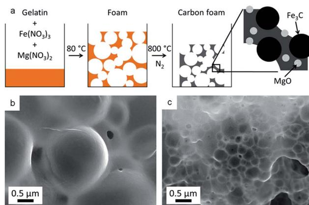
Fig. 1 (a) Schematic showing synthesis of carbon foam containing MgO and Fe<sub>3</sub>C nanoparticles from a gelatin precursor. Also SEM images showing foams made from (b) Fe(NO<sub>3</sub>)<sub>3</sub>/gelatin and (c) Mg(NO<sub>3</sub>)<sub>2</sub>/Fe(NO<sub>3</sub>)<sub>3</sub>/gelatin (at 75 : 25 molar ratio Mg : Fe).
