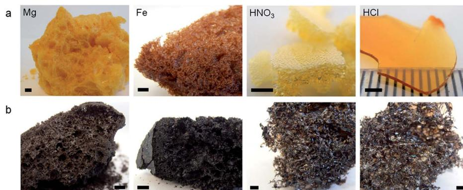
Fig. 2 Images of  $\text{Mg}(\text{NO}_3)_2/\text{gelatin}$ ,  $\text{Fe}(\text{NO}_3)_3/\text{gelatin}$ ,  $\text{HNO}_3/\text{gelatin}$ , and  $\text{HCl}/\text{gelatin}$  foams after (a) drying and (b) carbonization at 800 °C (scale bars 2 mm).
