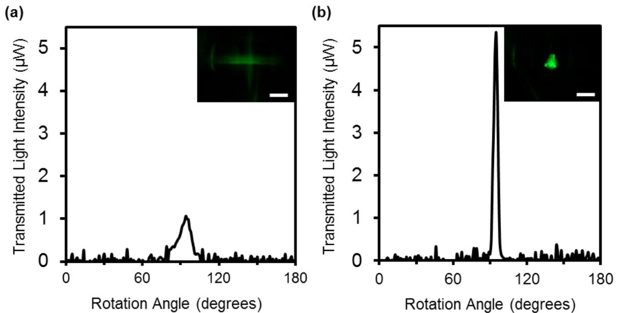
**Figure 5.** Transmitted light through the lattice structure having a mesh size of  $700 \mu\text{m}$ . Angle-resolved measurements of the transmitted light from the structure soaked with (a) diesel, and (b) stroke oil. The insets show the photographs of the transmitted light. Scale bars= 2 cm.
