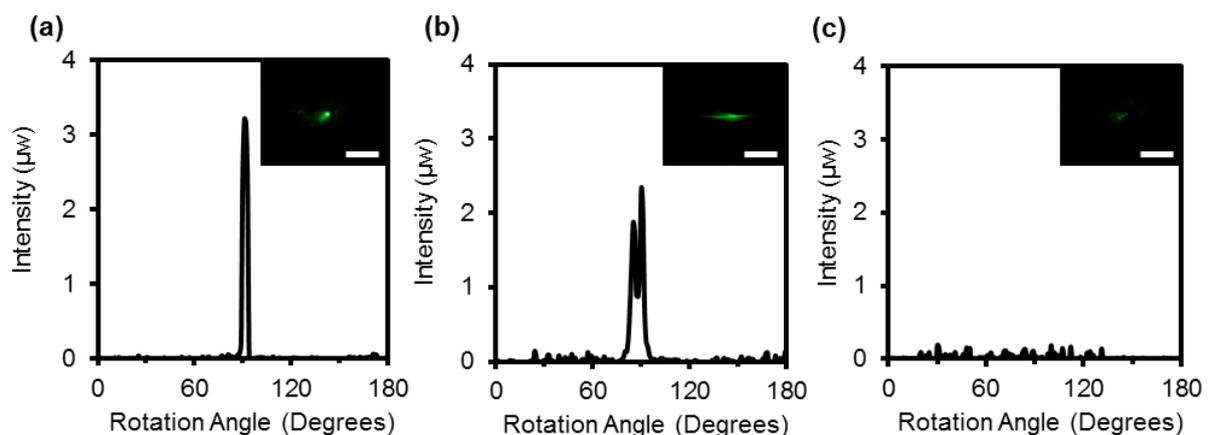
**Figure 4.** Transmitted light through the lattice structure having a mesh size of  $700 \mu\text{m}$ . Angle-resolved measurements of the structure having (a) air, (b) water, and (c) crude oil. (Scale bars= $1.5 \text{ cm}$ ).
