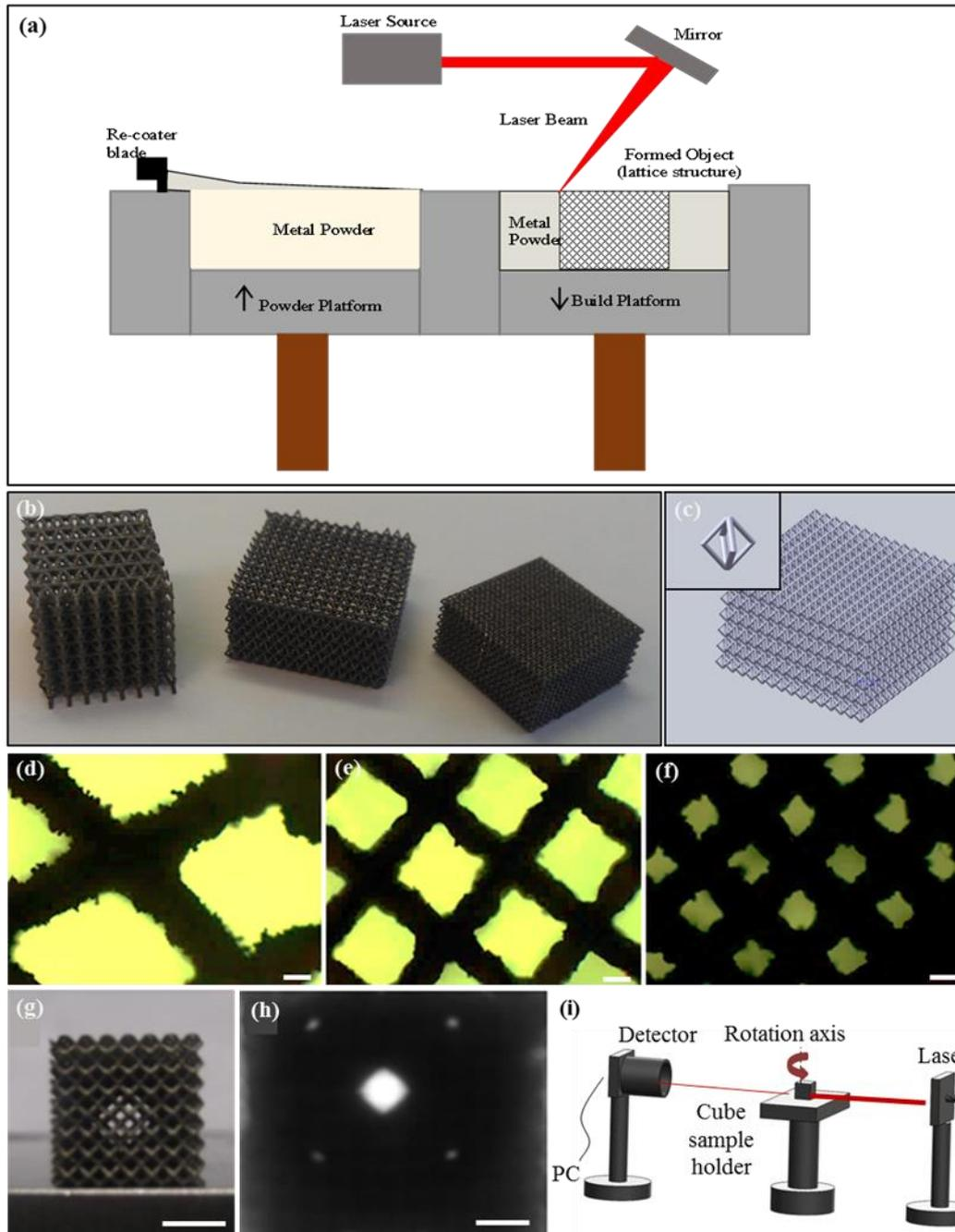
**Figure 1.** Fabrication of the 3D mesh structures. (a) Schematic of the selective laser melting process. (b) 3D-printed Ti-6Al-4V lattice for oil sensing mesh structures with the size of 1000, 700 and 400  $\mu\text{m}$  (scale bar=1cm). (c) Schematic view of the mesh structures. Optical
