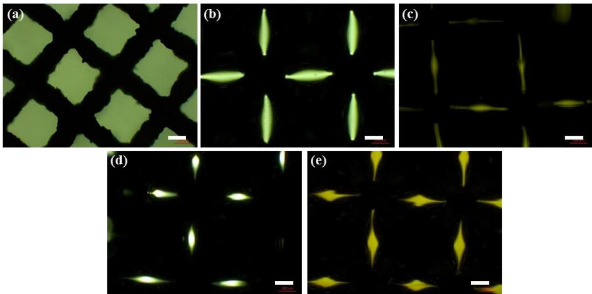
**Figure 3.** Transmittance optical images of lattice structures having a mesh size of 700  $\mu\text{m}$ . Mesh in the presence of (a) air, (b) water and (c) crude oil, (d) diesel, (e) stroke oil. (Scale bars = 200  $\mu\text{m}$ )
