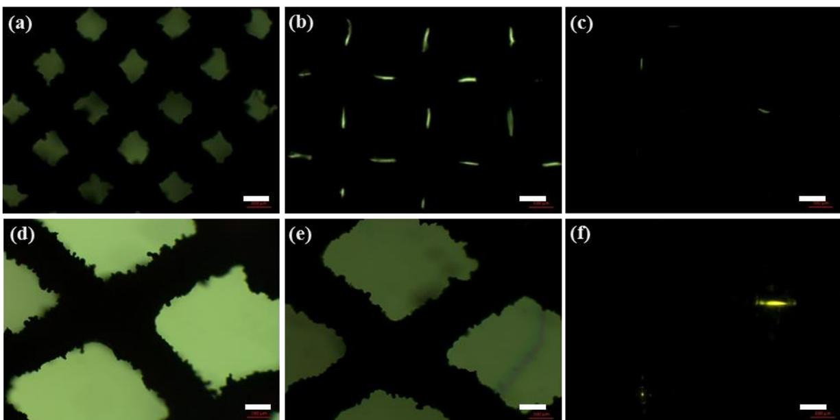
**Figure 2.** Transmitted light through 3D printed lattice structures. A lattice having a mesh size of 400  $\mu\text{m}$  in the presence of (a) air, (b) water, and (c) crude oil. A lattice having a mesh size of 1000  $\mu\text{m}$  under (d) air, (e) water, and (f) crude oil. Scale bars = 300  $\mu\text{m}$ .
