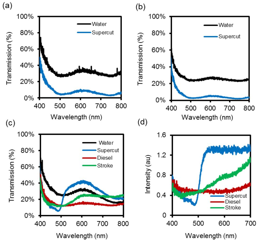
**Figure 6.** Spectroscopy measurements of the transmitted light through the mesh in the presence of different oil types. Crude oil measurements for (a) 400  $\mu\text{m}$ , (b) 1000  $\mu\text{m}$ , and (c) 700  $\mu\text{m}$ , where empty mesh was used as reference. (d) Transmission spectrum for 700  $\mu\text{m}$  considering the mesh with water as a reference.
