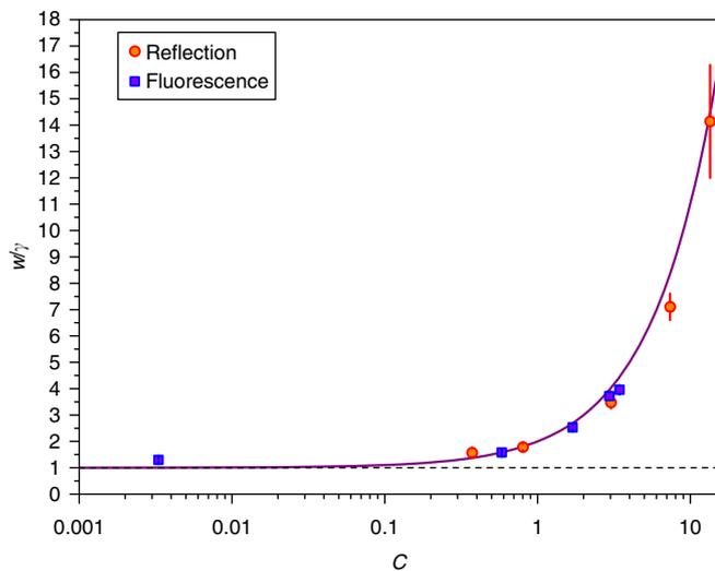
**Figure 5 | Measured resonance width  $w$  versus cooperativity  $C$ .** Data are extracted from the reflection and fluorescence spectra with  $\Delta_a = \Delta_c$ . The Lorentzian half-widths at half-maximum are normalized to the natural atomic line width  $\gamma$ , and error bars show the fit uncertainty. The dashed line is the asymptotic value  $\gamma$ , while the solid line shows the prediction  $w = \gamma(1 + C)$ .
