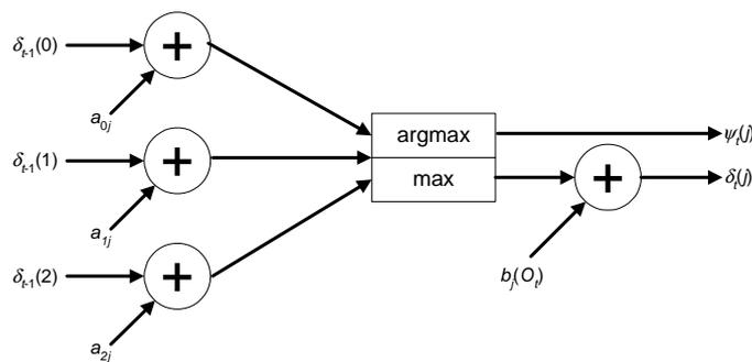
**Fig. 3.** Node structure. Each node processes the data corresponding to one state of an HMM. As every node depends only on the outputs of nodes produced in the previous time frame, and not the current one, the nodes can all be implemented in parallel
