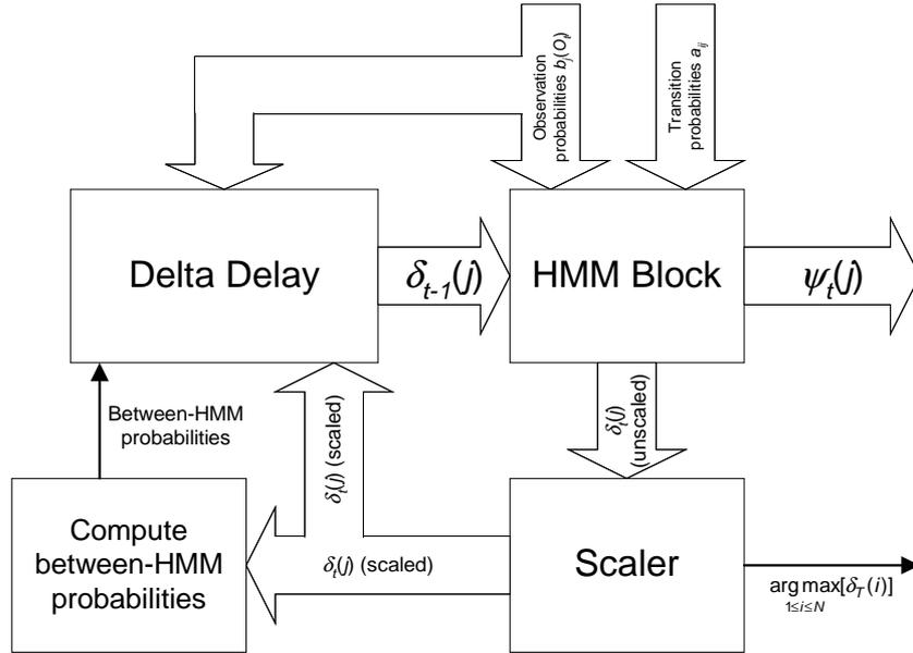
**Fig. 2.** System structure. The HMM Block contains the processing elements - nodes - which compute  $\delta_t(j)$ , the probability of the observation sequence up to time  $t$  and the “best” partial state sequence terminating in state  $j$  at time  $t$ ; and the most probable predecessors  $\psi_t(j)$
