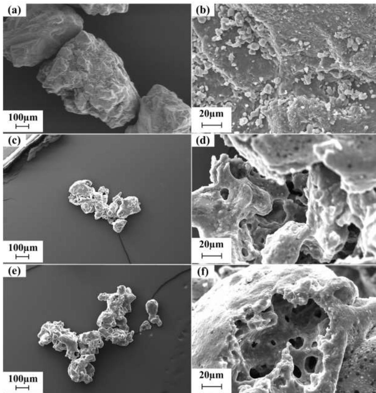
Figure 3. SEM images of particles at 100 and 1500 times magnification (a) (b)  $\text{Na}_2\text{CO}_3$  granules, (c) (d) PANDORA agglomerates 355-425  $\mu\text{m}$  size cut, and (e) (f) PANDORA agglomerates 425-600  $\mu\text{m}$  size cut.
