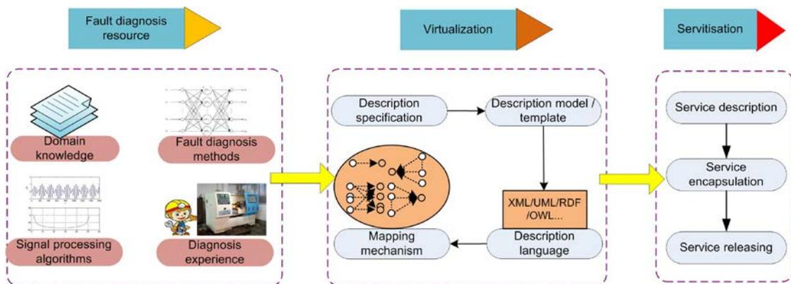
Fig. 2. Fault diagnostic methods virtualisation and servitisation
