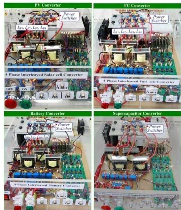
Fig. 12. Photograph of the implement converters.
