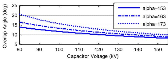
Fig. 5 Variation of overlap angle against capacitor voltage for different firing angles.
