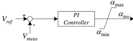
Fig. 10 Proposed Inverter AC voltage controller.
