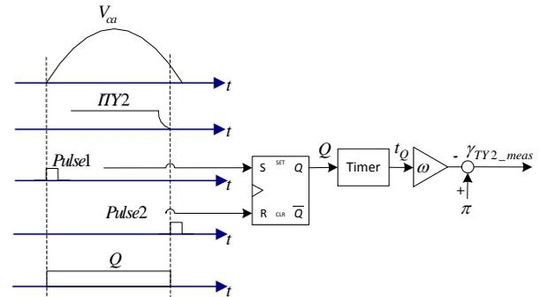
Fig. 8. Proposed extinction angle measurement for TY2.
