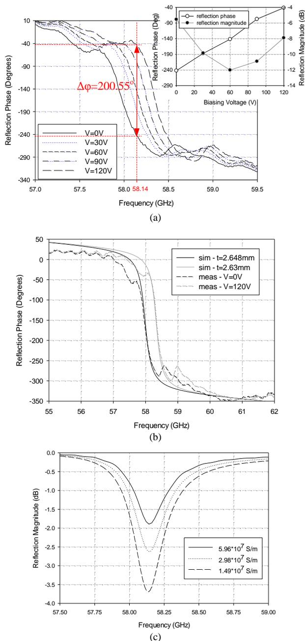
Fig. 4. (a) Measured reflection magnitude and reflection phase for different voltages, (b) Comparison of simulated and measured reflection phase for  $V=0V$  and  $V=120V$  and (c) Simulated reflection magnitude for  $t=2.64mm$  for different copper conductivity values.
