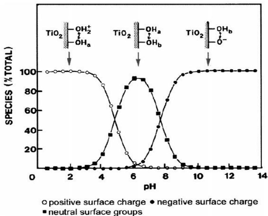
Fig.4 Concentration of the different charged and uncharged hydroxy-related species at a titanium oxide surface (%) as a function of pH of the aqueous solution.  $-\text{OH}_a$  and  $-\text{OH}_b$  denote acidic and basic hydroxyl group (adapted from [71]), respectively.
