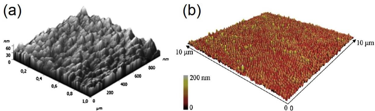
Fig. 7 AFM images showing the nano-structures that exhibit antibacterial properties. (a) TiO<sub>2</sub> nanopores with 15nm diameters using anodization (adapted from Krunal et al. [149]), (b) Cicada wing structure (adapted from Pogodin et al. [152]).
