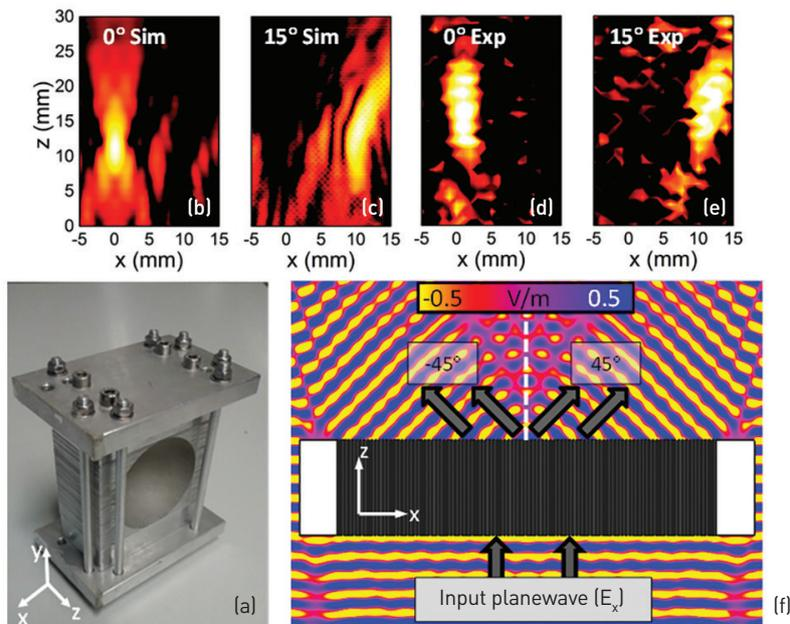
(a) Fabricated planoconcave ENZ lens. (b-c) Simulation and (d-e) experimental results of the normalized transmission under normal (b, d) and oblique (c, e) incidence. (f) Simulation results for the  $E_x$ -field on the  $xz$ -plane for an ENZ-GRIN power splitter designed to deflect an incoming plane wave to  $\pm 45^\circ$  at its output.
