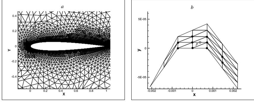
**Fig. 1** (a) An unstructured computational grid generated about an airfoil. (b) A reconstruction stencil for LS approximation at a given edge midpoint. Grid points used to reconstruct the solution at point  $p$  are shown as closed black circles in the figure. Note a different length scale along the  $x$  and  $y$ -axes.
