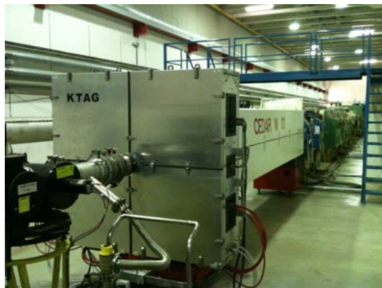
Figure 14: The environmental chamber enclosing KTAG is shown in its final position on the beam line as part of the NA62 experiment in the North Area at CERN. The CEDAR gas enclosure can be seen behind KTAG.
