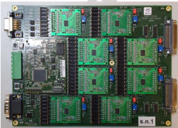
Figure 15: Prototype front-end board for 2012 run, equipped with 8 NINO mezzanines.
