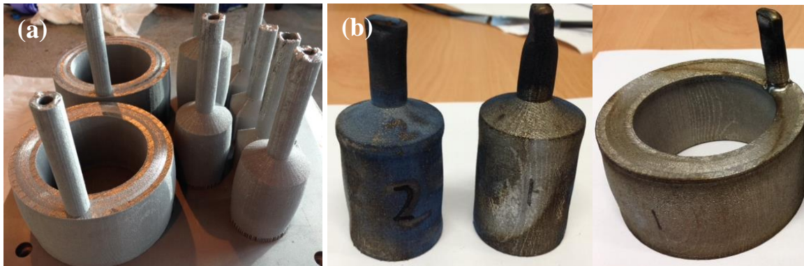
Fig. 3 Photographs showing several tooling designs (a) before and (b) after HIPing
