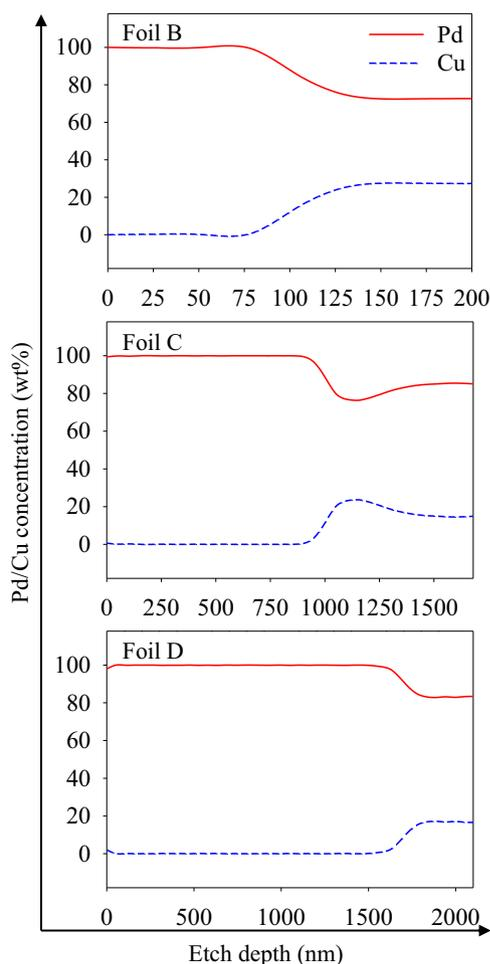
**Fig. 4.** XPS depth profile analysis of Foils B–D in the as-deposited state.
