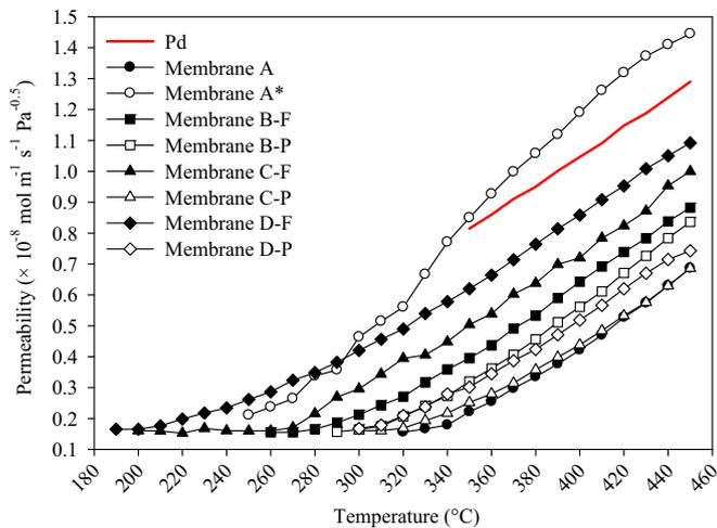
**Fig. 5.** Hydrogen permeability as a function of temperature plot comparing each membrane investigated in this work. All curves, except Membrane A\*, show the heating stage of the initial third cycle completed by each membrane between 50 and 450 °C using a hydrogen feed pressure of 445 kPa and permeate pressure of 100 kPa. The Membrane A\* curve represents the third cycle completed between 250 and 450 °C following the completion of two cycles between 250 and 700 °C.
