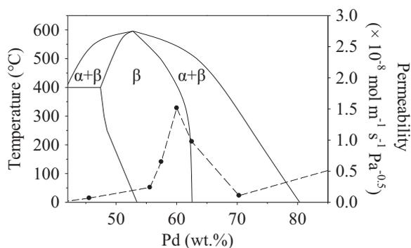
**Fig. 1.** Pd–Cu phase diagram where ‘ $\alpha$ ’ denotes the FCC phase and ‘ $\beta$ ’ denotes the BCC phase. The phase diagram has been reproduced from literature [13,17] and also features a hydrogen permeability dashed line plot as a function of Pd content at 350 °C compiled using data from Howard et al. [15].
