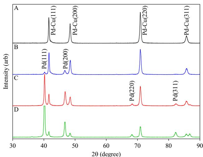
**Fig. 3.** XRD patterns acquired for Membrane A and the Pd sputter coated surfaces of Membranes B–D in the as-deposited state prior to MPR testing which indicate a single phase FCC crystal structure present in the bulk Pd–Cu membranes. The FCC Pd diffraction peaks shown in patterns B, C and D indicate the presence of the Pd thin film in Membranes B, C and D, respectively.
