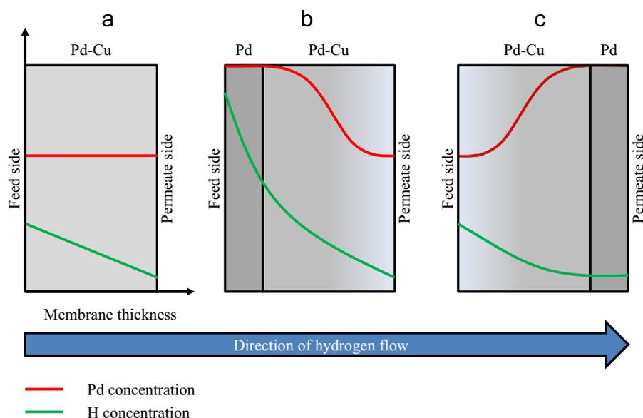
**Fig. 8.** A schematic illustration showing Pd and H concentration as a function of membrane thickness during MPR testing at a given temperature where (a) represents Membrane A, (b) represents Membranes B-F, C-F and D-F; and (c) represents Membranes B-P, C-P and D-P.
