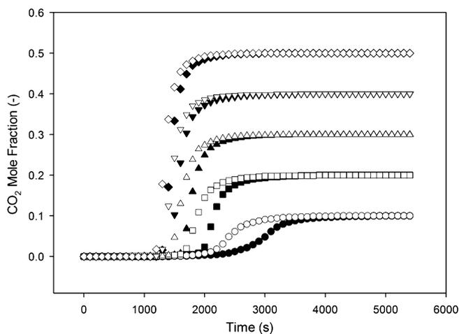
**Figure 4.** Breakthrough curves for the separation of a CO<sub>2</sub>/N<sub>2</sub> mixture using unmodified activated (black) compared to the modified activated carbon material (white).
