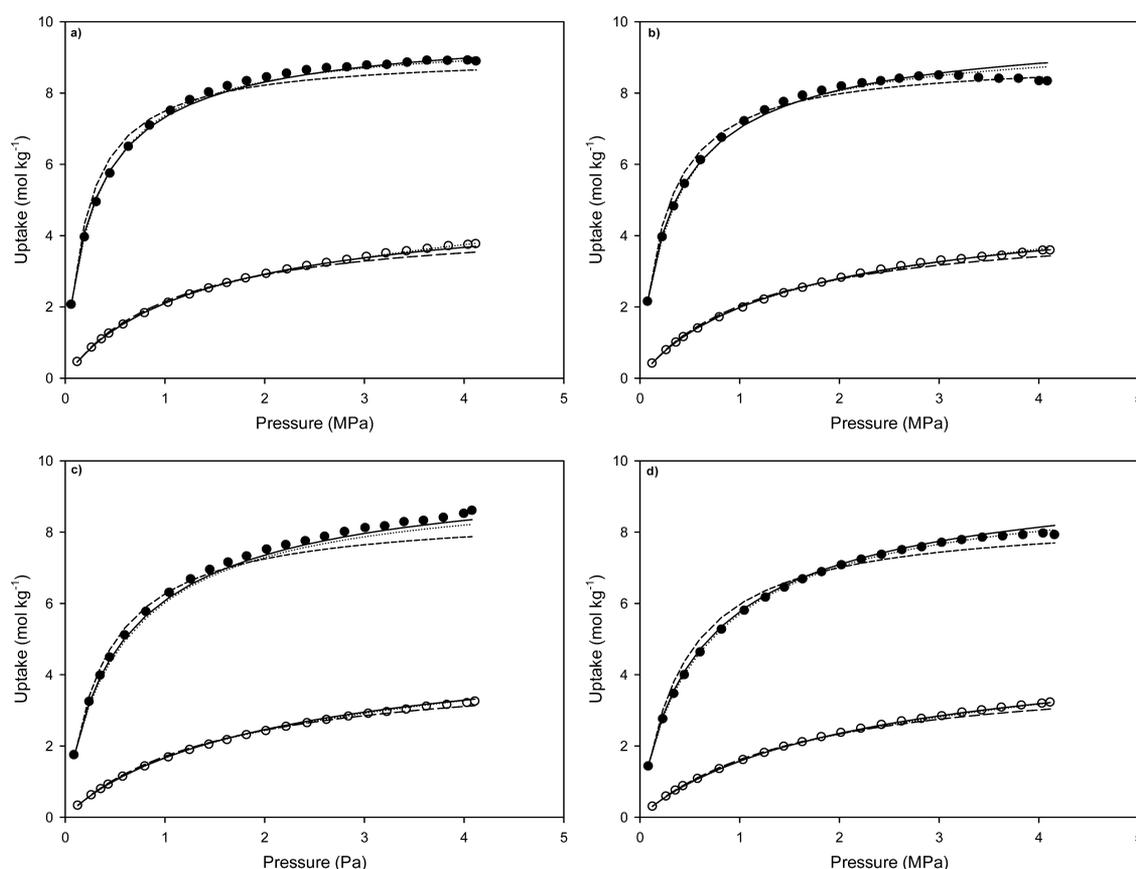
**Figure 3.** Experimental isotherms for modified activated carbon for CO<sub>2</sub> (●) and N<sub>2</sub> (○) at (a) 25 °C, (b) 30 °C, (c) 45 °C, and (d) 50 °C and their corresponding isotherm equations: Langmuir (---), LF (—), and DSL (⋯).
