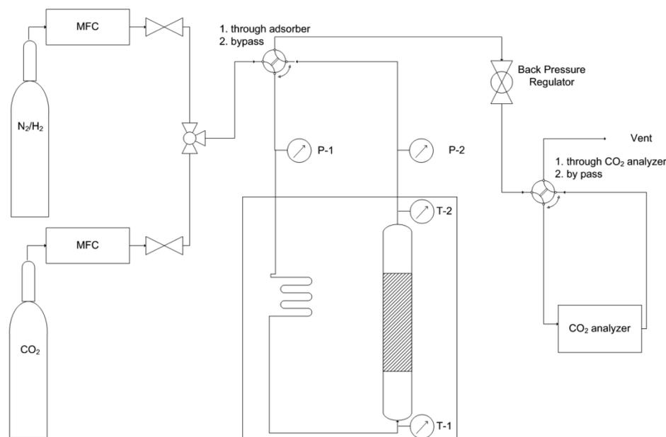
Figure 1. Experimental setup of the fixed-bed adsorption rig.
