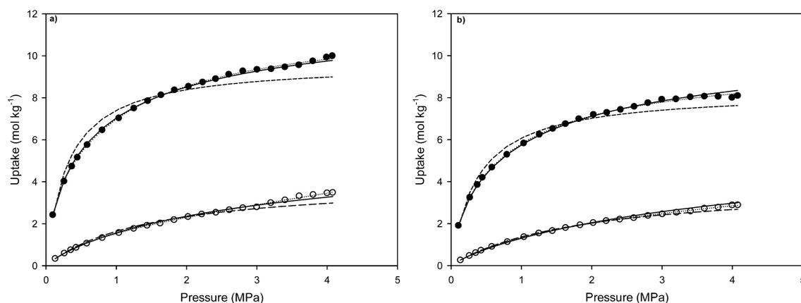
**Figure 2.** Experimental isotherms for unmodified activated carbon for CO<sub>2</sub> (●) and N<sub>2</sub> (○) at (a) 30 °C and (b) 45 °C and their corresponding isotherm equations: Langmuir (---), LF (—), and DSL (⋯).
