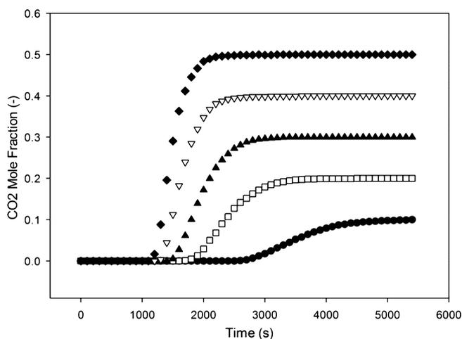
**Figure 6.** Breakthrough curves for the separation of a CO<sub>2</sub>/H<sub>2</sub> mixture using modified activated carbon at CO<sub>2</sub> feed fractions of 0.1 (●), 0.2 (□), 0.3 (▲), 0.4 (▽), and 0.5 (◆).
