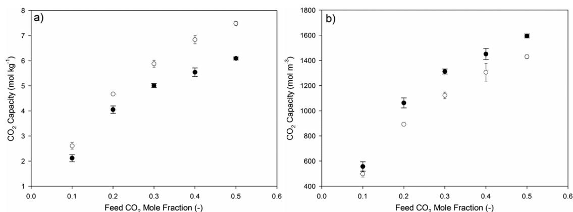
**Figure 5.** Comparison of unmodified (●) and modified (○) activated carbon breakthrough capacities for the separation of CO<sub>2</sub>/N<sub>2</sub> mixtures on (a) mass and (b) volumetric basis.
