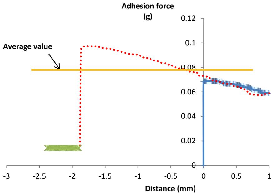
Figure -4 A typical submersion – retraction curve for wax A,  $\alpha$  to  $\beta$   $\rightarrow$  showing submerging of samples into wax,  $\beta$  to  $\chi$   $\rightarrow$  is emerging and  $\delta$  to  $\epsilon$   $\rightarrow$  plateau of weight after lifting. It shows the advancing and receding force of wax A in this case did not have any obvious hysteresis behaviour. The horizontal orange line shows the averaged adhesion tension value
