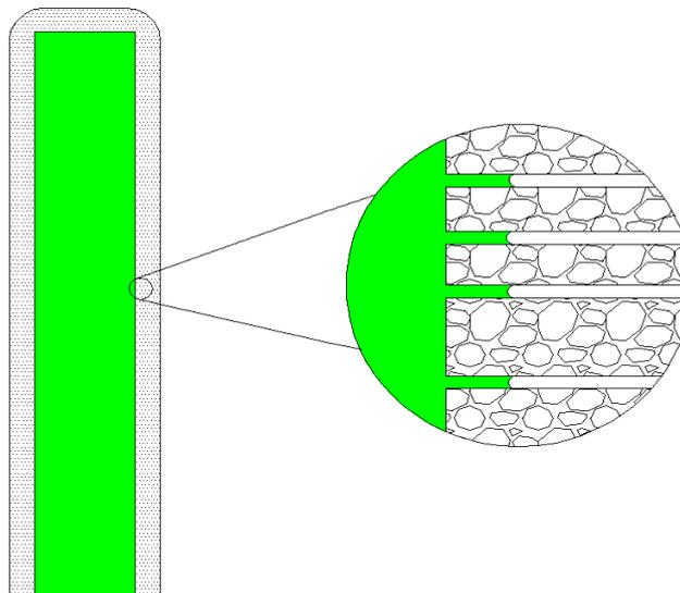
15 **Figure-1 Schematic representation of the initial de-waxes process where wax is forced into the porous ceramic shell. In the models where Poiseuille is assumed, the pores are represented as horizontal tubes**
