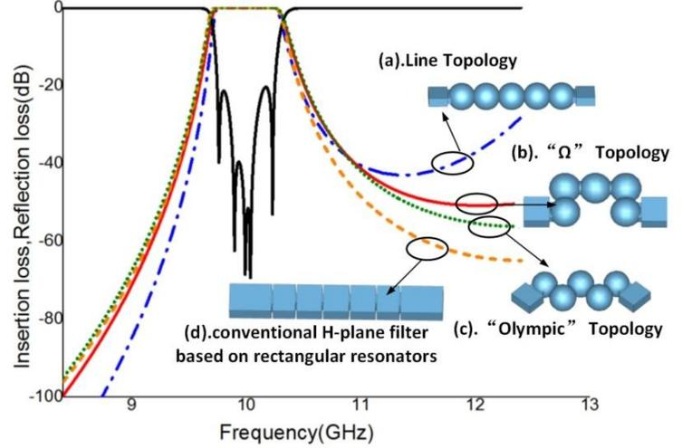
Fig.3. Simulation results of the filters with different topologies: (a) Line topology without any higher modes rejection mechanisms; (b) ‘‘ $\Omega$  topology’’ with considerable rejection and it is utilized in this work; (c) ‘‘Olympic topology’’ with the best rejection; (d) A H-plane filter based on rectangular resonators
