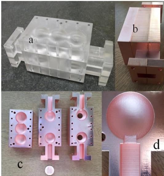
Fig. 4. Photographs of the filter before and after plating. (a) Before plating; (b) and (c) after plating; (d) enlarged view of one spherical resonator.
