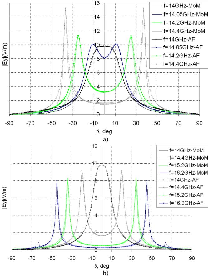
Fig. 9 Radiation pattern a) H-plane and b) E-plane of the LWA with dimensions (in mm)  $D=9.0$ ,  $h=3.25$ , for the PRS: square patches  $L_{PRS}=8$ ,  $h_{d1}=1.5$  and  $\epsilon_r=2.55$  and for the AMC: square patches  $L_{AMC}=4.3$ ,  $h_{d2}=1.15$  and  $\epsilon_r=2.2$  operating at 14GHz as obtained using Full-wave MoM and Array Factor procedure.
