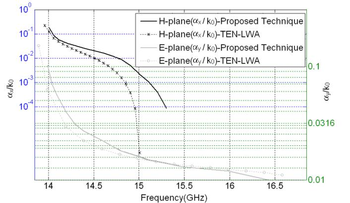
Fig. 8. Normalized leakage rate versus frequency for the H-plane and E-plane as obtained by the proposed technique and a Transverse Equivalent Network for the sub-wavelength antenna of Fig. 7.
