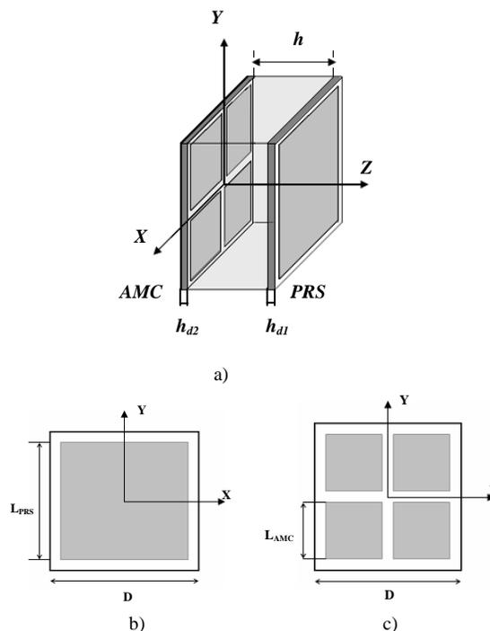
Fig. 1. a) Layout of the resonant cavity leaky-wave antenna formed by metalodielectric PRS and AMC with excitation source inside the cavity b) Unit cell of a square patch PRS array and c) AMC array.
