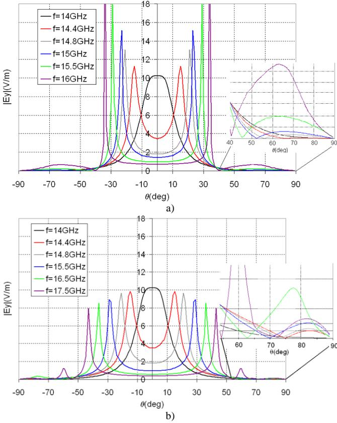
Fig. 3 Radiation pattern a) H-plane and b) E-plane of the LWA formed with a square patch PRS with dimensions (in mm)  $D=9.0$ ,  $L_{PRS}=8$ ,  $h_{dl}=1.5$ ,  $h=9.82$  and  $\epsilon_r=2.55$ .
