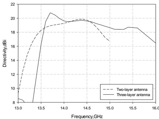
Fig. 7. Directivity comparison between three-layer and two-layer antenna.
