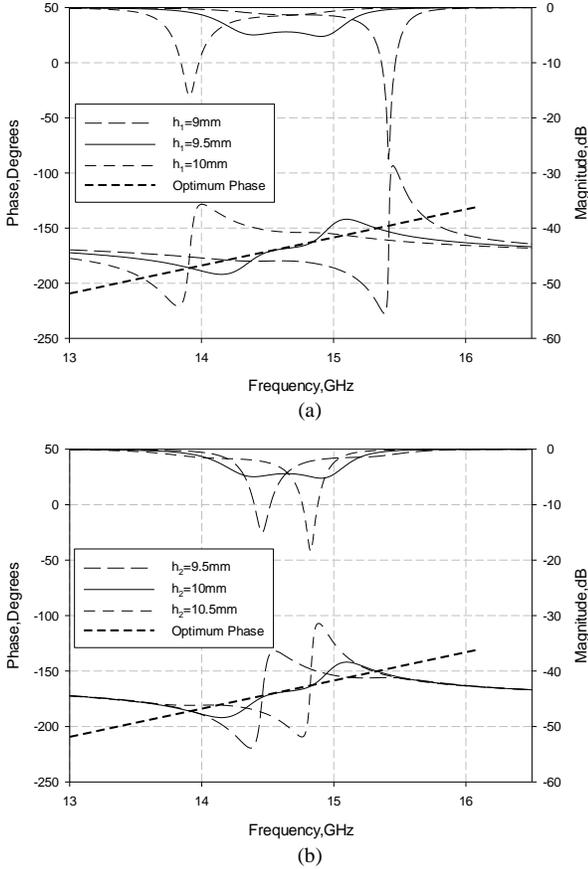
Fig. 5. Complex Reflection Coefficients of the three-layer PRS changing (a) the cavity distance  $h_1$  ( $h_2=10\text{mm}$ ,  $d_1=9.16\text{mm}$ ,  $d_2=10\text{mm}$ ,  $d_3=6\text{mm}$ ), (b) the cavity distance  $h_2$  ( $h_1=9.5\text{mm}$ ,  $d_1=9.16\text{mm}$ ,  $d_2=10\text{mm}$ ,  $d_3=6\text{mm}$ ).
