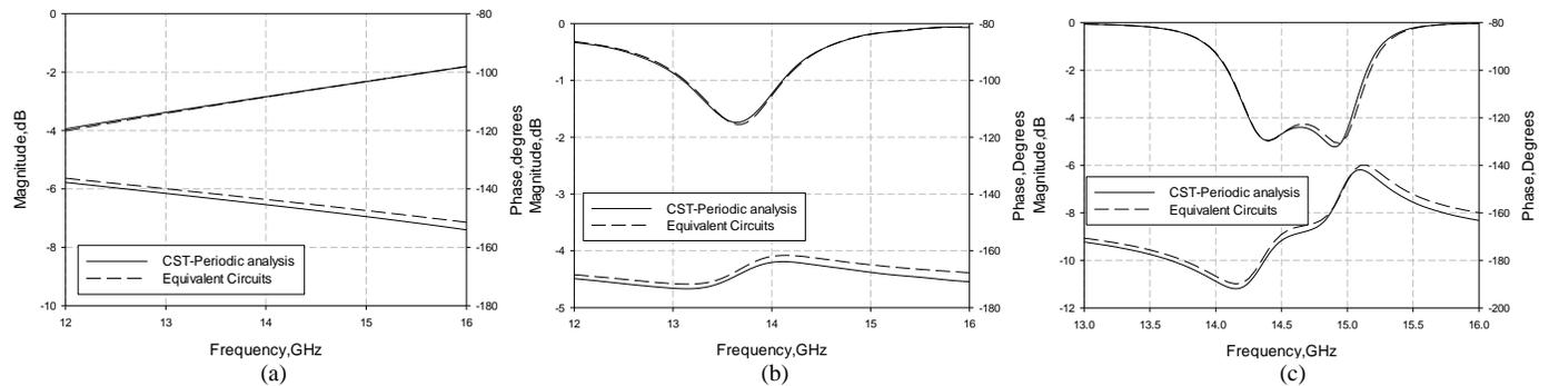
Fig. 3. Complex Reflection Coefficients for (a) single-layer PRS for  $d=6\text{mm}$ , (b) double-layer PRS for  $d_1=10\text{mm}$ ,  $d_2=6\text{mm}$  and  $h_1=11\text{mm}$ , (b) three-layer PRS for the proposed design dimensions, obtained from the equivalent circuit model and periodic full-wave analysis.
