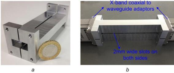
**Fig. 4** Photograph of the fabricated X-band filter.
