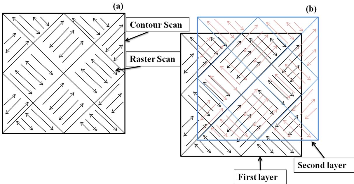
**Figure 2 Schematic illustration of the island scan strategy, showing (a) each layer is divided into square (islands) and the inside of island is raster scanned, then (b) the successive layers are displaced 1 mm in the X and Y-directions.**
