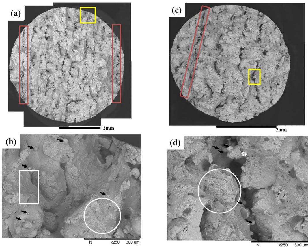
**Figure 10** Backscattered SEM fractographs of SLM fabricated AlSi10Mg horizontal samples, showing (a) RT tensile test sample, (b) enlarged image, shown in yellow square in (a), (c) Creep test sample, tested at 180°C/200 MPa and (d) enlarged image, shown in yellow square in (c). Dimples-containing areas are circled, and the smooth areas are labelled using white rectangles. Unmelted particles are arrowed.
