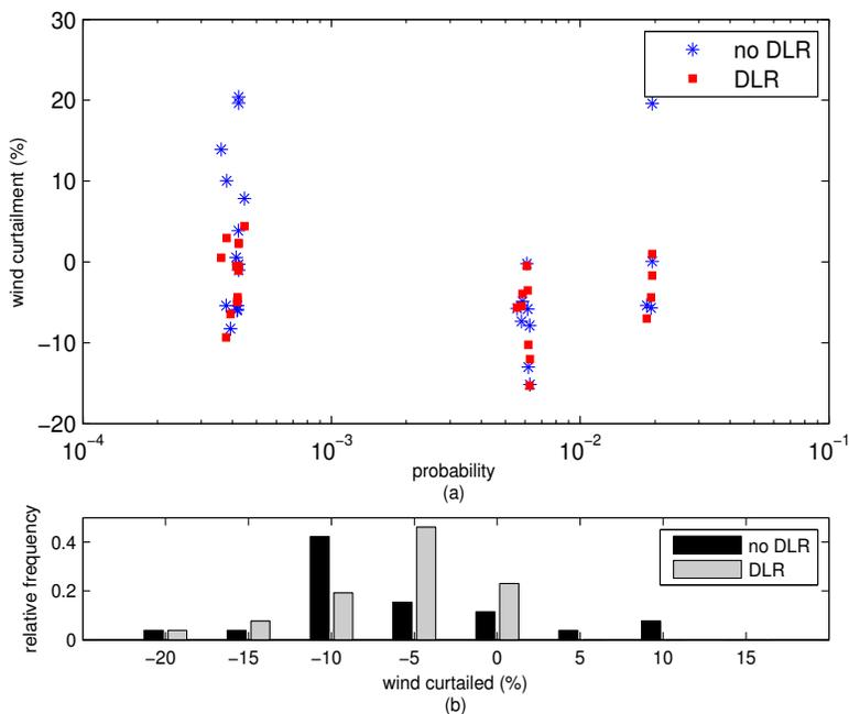
Fig. 7 (a) Post outage wind curtailment profile for 118 bus system (b) Histogram of post outage wind curtailment
