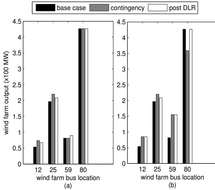
Fig. 9 Wind power generation profile for outage in (a) branch between bus 23 – 25 (b) branches between bus 64 – 65 and 38 – 65
