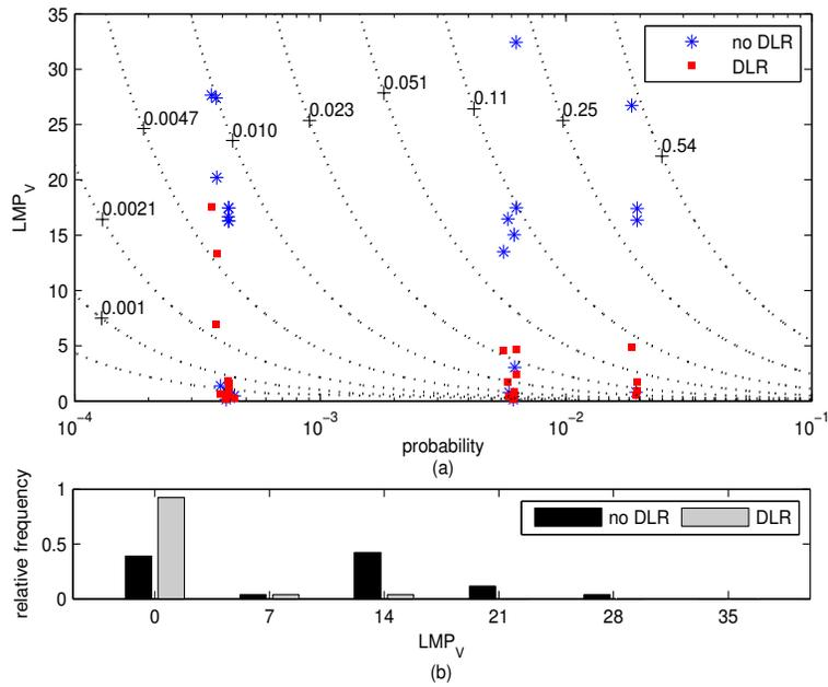
Fig. 8 Comparison of post outage risk profile of 118 bus system with and without DLR
