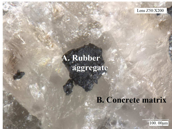
(c) Rubber-matrix interface of CRC20
