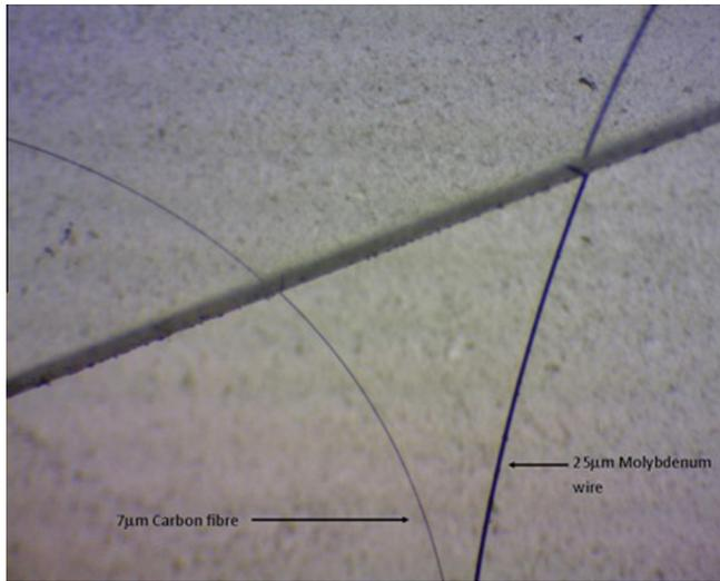
**Fig. 3.** Single carbon fibre with 25 µm Molybdenum wire for scale (optical microscope) (For interpretation of the references to colour in this figure legend, the reader is referred to the web version of this article.).
