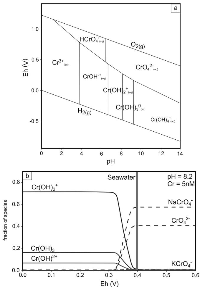
**Fig. 1.** (a) Speciation of Cr in seawater as a function of Eh and pH. (b) Relative proportion of different Cr species in seawater as a function of Eh, where pH = 8.2. Calculations were undertaken using Geochemists Workbench, for a total Cr concentration of 5 nM.
