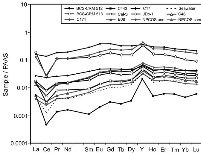
**Fig. 4.** Shale-normalised REE-Y patterns of modern-day (B08, NPCOS cem, NPCOS unc, C48) and Phanerozoic carbonates. Seawater is shown for comparison, although the concentrations have been multiplied by 10000. Shale values from Taylor and McLennan (1985).
