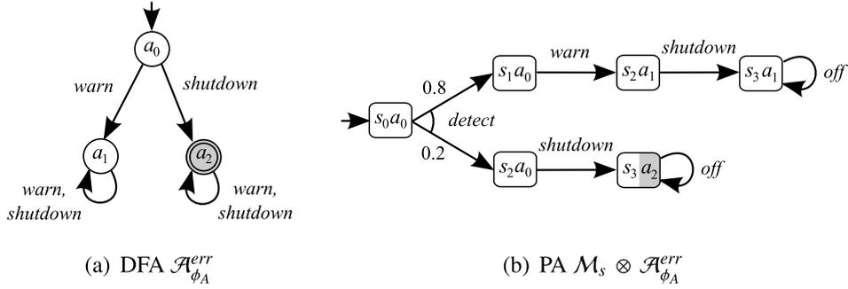
Fig. 3. A DFA  $\mathcal{A}_{\phi_A}^{err}$  for safety property  $\phi_A$  and the product  $\mathcal{M}_s \otimes \mathcal{A}_{\phi_A}^{err}$  (see Example 3).
