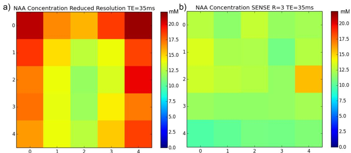
FIG. 3. NAA concentration map for a phantom calculated from reduced resolution water reference data (a) and SENSE ( $R=3$ ) water reference data (b) for the central  $5 \times 5$  voxel region. [Color figure can be viewed in the online issue, which is available at [wileyonlinelibrary.com](http://wileyonlinelibrary.com).]
