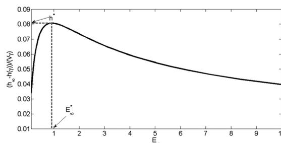
**Fig. 9** Determination of optimality  $E_\infty^*$ : for the typical hydrogel properties obtained from Table 4 and the system parameters in Table 5 except  $\gamma = 0.1$  s and the spring stiffness which is varied. The grey dashed line (---) represents the optimal  $E_\infty^* = 0.916$  corresponding to a spring stiffness of  $0.549 \text{ N m}^{-1}$  and the maximum relative relaxation depth,  $h^* = 0.0807$ .
