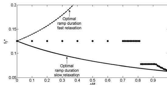
**Fig. 11** Optimal ramp duration as a function of the normalised frequency difference is represented by the solid markers. The solid line represents the optimal ramp duration for the slow relaxation time,  $\tau_1$ . The dashed line (---) represents the optimal time for the fast relaxation,  $\tau_2$ .
