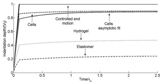
**Fig. 7** Comparison of the indentation depth as a function of time for the various materials; the black solid line (—) represents the motion of the fixed end; the cells represented by the dashed line (---) were obtained by the numerical code, the solid grey line (—) is the asymptotic fit to eqn (S1.6); the grey dotted line (...) is the hydrogel and the grey dot dashed line (-.-) is the elastomer obtained numerically.
