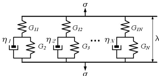
**Fig. 4** Schematic of standard linear solid model.  $\eta_n$  is the viscosity of the damping component (dashpot),  $G_{1n}$  and  $G_n$  are the elastic moduli of the restorative force components (springs),  $\alpha$  and  $\lambda$  are the stress and strain applied to the element respectively.
