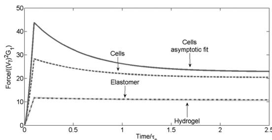
**Fig. 8** Comparison of the indentation force as a function of time for the various materials; the cells represented by the grey dashed line (---) were obtained by the numerical code, the solid grey line (—) is the asymptotic fit to eqn (S1.6); the grey dotted line (...) is the hydrogel and the grey dot dashed line (-.-) is the elastomer obtained numerically.
