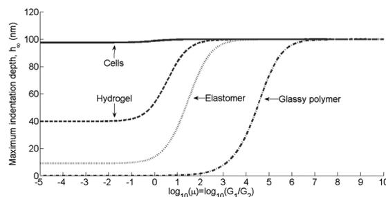
**Fig. 5** Variations in the maximum indentation depth provided by eqn (7) as  $G_2$  is varied for a Prony series with  $N = 2$ . Low  $\mu$  values correspond to the elastic limit and high  $\mu$  values correspond to the Maxwell limit. The material parameters  $G_1$  and  $\tau$  are given in Table 4 and the system parameters are supplied in Table 5.
