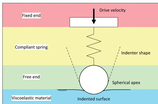
Fig. 1 Standard elements present during an indentation measurement.
