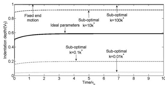
**Fig. 13** Indentation curves for the hydrogel with a ramp duration of 0.1 s and the following ideal parameters  $V = 17 \mu\text{m s}^{-1}$ ,  $R = 10 \mu\text{m}$  and  $k^* = 8 \text{N m}^{-1}$ , where the spring constant is altered as specified for the sub-optimal cases.
